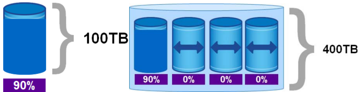
Figure 82 Converting a FlexVol volume that is nearly full and at maximum capacity
