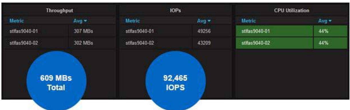
Figure 73 Average CPU utilization, throughput, and IOPS for a FlexGroup volume—ETERNUS AX4100 HA pair, 128 threads
