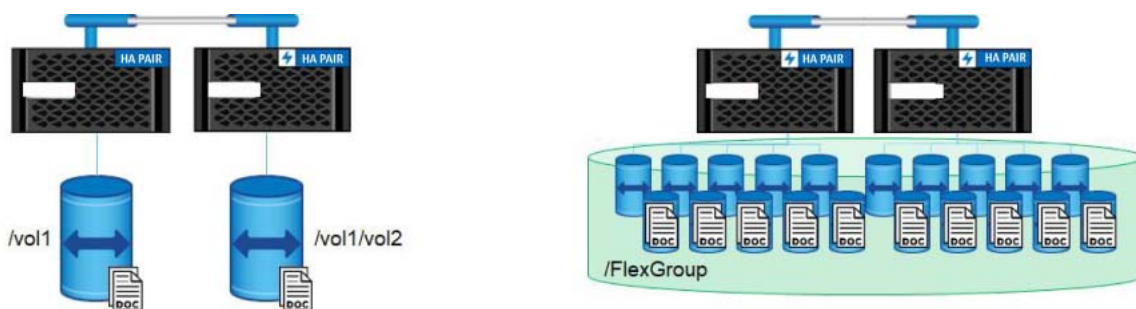
Figure 19 FlexVol and FlexGroup architecture comparison
