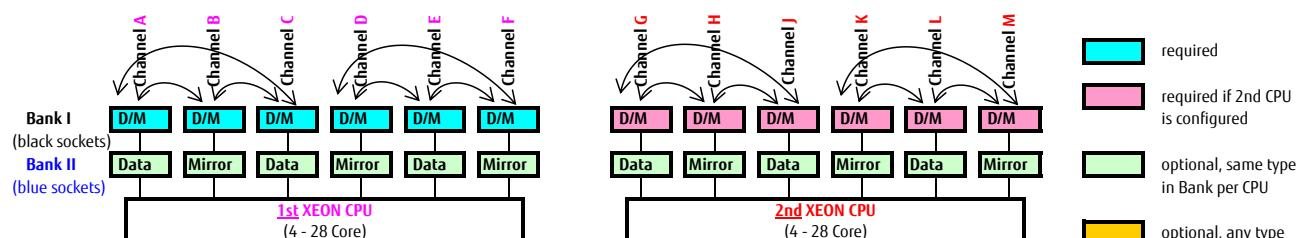
Mirrored Channel Mode requires identical modules on channel A, B, C, D, E, F (1st CPU) or channel G, H, J, K, L and M (2nd CPU) 50% of the capacity is used for the mirror => the available memory for applications is only half of the installed memory. If this mode is used, a multiple of 6 identical modules has to be ordered.
