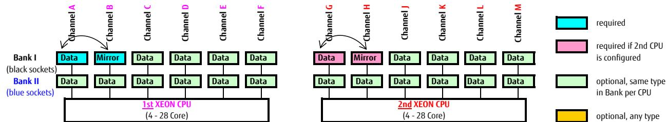
Mirrored Channel Mode (2 DIMMs per CPU) requires identical modules on channel A & B (1st CPU) or channel G & H (2nd CPU) 50% of the capacity is used for the mirror => the available memory for applications is only half of the installed memory. If this mode is used, a multiple of 2 identical modules has to be ordered.
