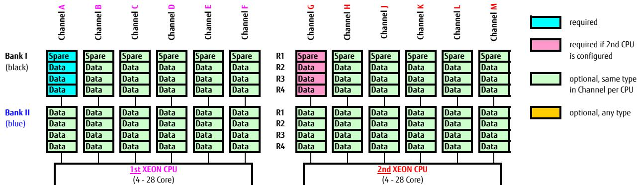
Rank Sparring Mode requires identical modules (same capacity and technology) within the same channel. The available memory for applications will vary depending on configuration. Please refer to the spreadsheet above "Effective Memory capacity with active Rank Sparring Mode". Population rule for Rank sparing mode is to achieve max. available memory, e.g. 4 DIMMs will be spread across two channels, each with 2DPC.
