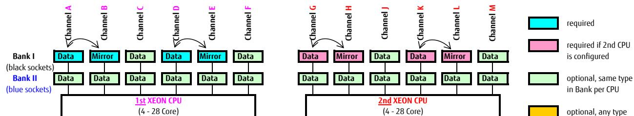
Mirrored Channel Mode (4 DIMMs per CPU) requires identical modules on channel A, B, D & E (1st CPU) or channel G, H, K & L (2nd CPU) 50% of the capacity is used for the mirror => the available memory for applications is only half of the installed memory. If this mode is used, a multiple of 4 identical modules has to be ordered.
