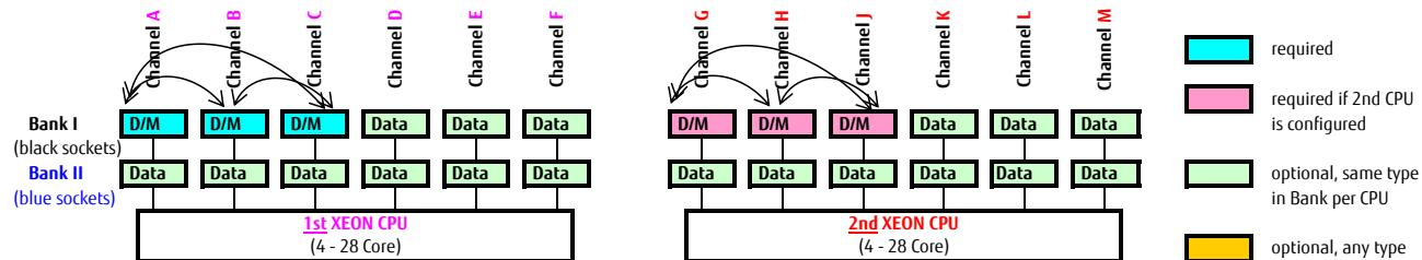
Mirrored Channel Mode (3 DIMMs per CPU) requires identical modules on channel A, B & C (1st CPU) or channel G, H & J (2nd CPU) 50% of the capacity is used for the mirror => the available memory for applications is only half of the installed memory. If this mode is used, a multiple of 3 identical modules has to be ordered.
