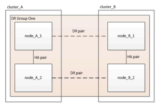
At the conclusion of this procedure, the MetroCluster FC configuration consists of two HA pairs at each site:
