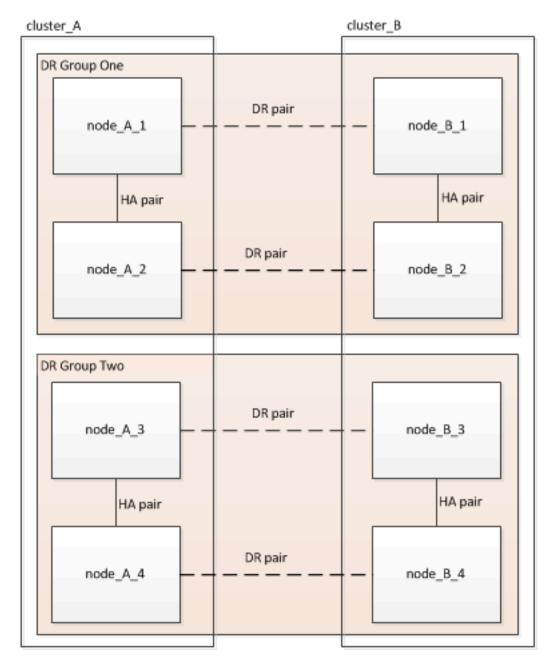
Both sites must be expanded equally. A MetroCluster FC configuration cannot consist of an uneven number of nodes.
