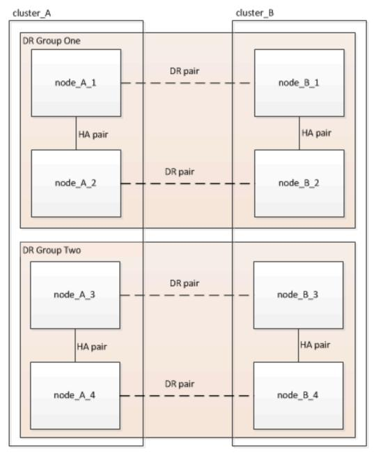
By removing a DR Group, four nodes remain in the configuration.
