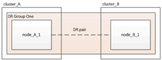
After completing this procedure, the MetroCluster FC configuration consists of two HA pairs, one at each site:
