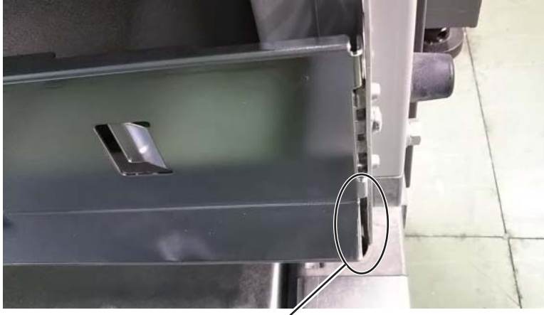
The rack rail hook is on the edge of the adapter block
