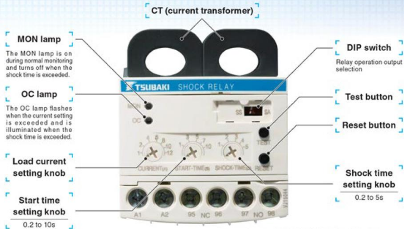
* Picture shows the SHOCK RELAY with the DIP switch cover removed.
