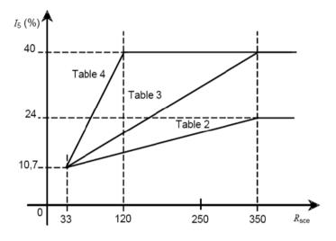
Figure A.1 – Limits of the 5<sup>th</sup> harmonic current as functions of  $R_{sce}$
