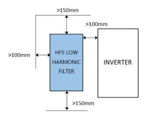
Install the product in consideration of the access space for removing the front cover when inspecting and maintaining the product.
