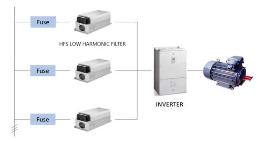
An application, having one HFS harmonic filtering harmonics of several drives, requires in any case line side fuse protection of the drives as well as the correct filter protection.
