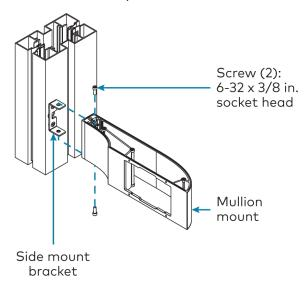
8. Align the TSW-770/TSW-1070 mounting bracket (included with touch screen) with the panel cover as shown in the illustration below, and then secure both to the mullion mount with the four 4-40 x 1/2 in. undercut head screws.
