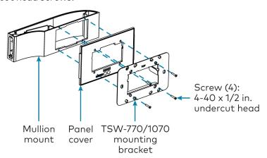
If the TSW-770-LB or TSW-1070-LB light bar will be used in this installation, the light bar should be placed in between the TSW-770/1070 mounting bracket and the panel cover as shown in the illustration below.
