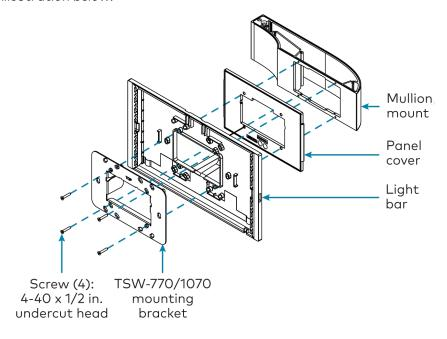
9. Reattach the two fitted cover plates on the top and bottom of the mullion mount so that the cover plates magnetically snap into place against the exposed screws.
