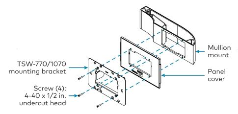
If the TSW-770-LB or TSW-1070-LB light bar will be used in this installation, the light bar should be placed in between the TSW-770/1070 mounting bracket and the panel cover as shown in the illustration below.
