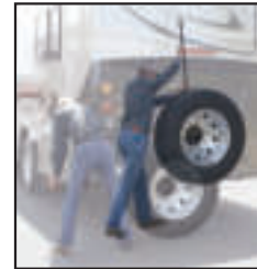
The pivot bolt acts like a fulcrum, allowing you to easily raise or lower the tire with the included lever arm.
