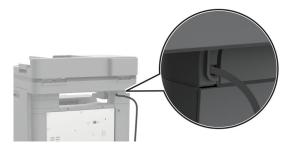
11 Connect the stapler and the printer power cords to the electrical outlet, and then turn on the printer.
