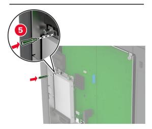
**5** Attach the controller board shield.
