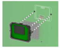
**6** Attach the controller board shield.
