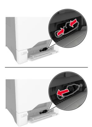
**4** Apply isopropyl alcohol to a soft, lint-free cloth, and then wipe the pick roller.
