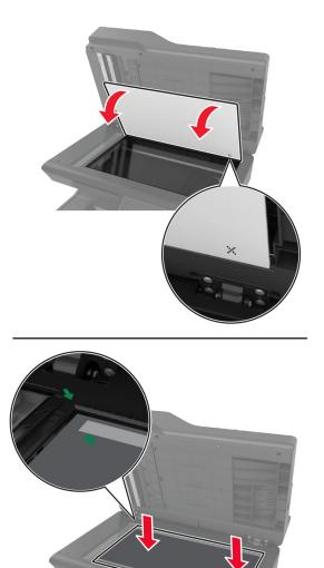
**Note:** Make sure that the scanner glass pad is aligned correctly on the edges of the scanner glass.
