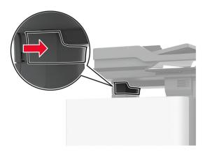
**7** Insert the power supply through the printer.
