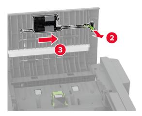
**3** Remove the ADF separator roller.
