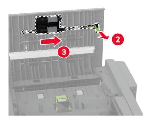
Remove the used ADF separator roller.
