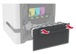
**Note:** To avoid spilling the toner, place the bottle in an upright position.
