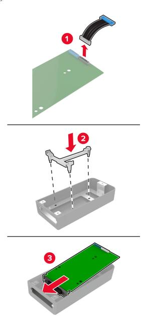
Attach the housing to the controller board shield.
