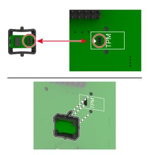
**6** Attach the controller board shield.
