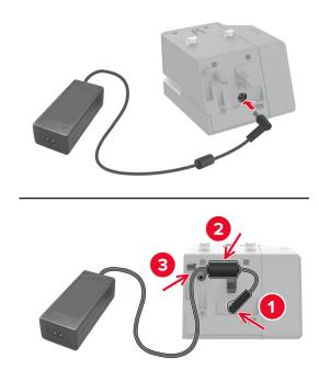
**Note:** Use only the power supply that came with the convenience stapler. Using any other power supply can damage the product.
