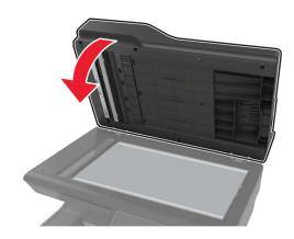
**6** Open the scanner cover to check if the new scanner glass pad is properly attached to the cover.
