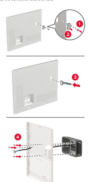
Connect the wireless assembly to the ISP connector in the controller board.
