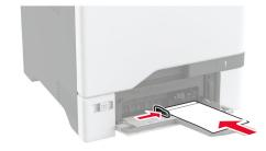
**Warning—Potential Damage:** Do not use envelopes with stamps, clasps, snaps, windows, coated linings, or self-stick adhesives.
