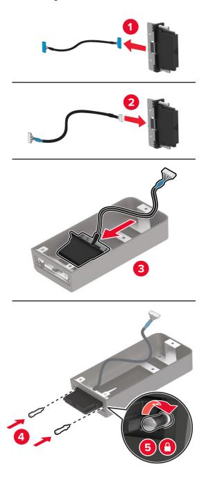
Attach the wireless module to the controller board shield.
