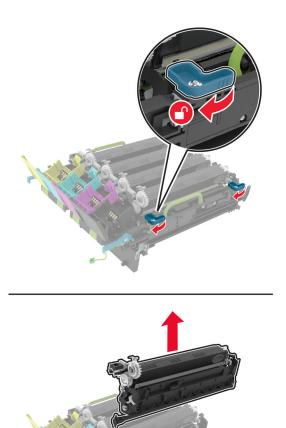
**Warning—Potential Damage:** Do not expose the photoconductor unit to direct light for more than 10 minutes. Extended exposure to light may cause print quality problems.
