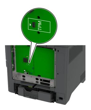
Attach the module to the TPM connector.
