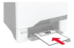
• Load envelope with the flap side up and against the right side of the paper guide. Load European envelopes with the flap entering the printer first.
