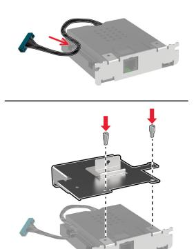
Install the fax card and attach the connector to the controller board.
