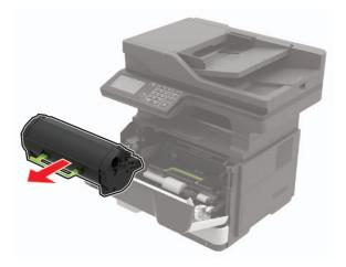
Remove the used imaging unit.
