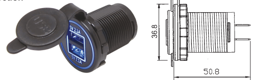
K32203 USB/A & C type charger W/fuse W/reverse / short circuit / over voltage protection W/LED / voltage & current meter In:12V/24V Out:5V 2.4A
