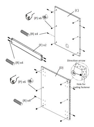
4. Drop Rack Top (C), Rack Bottom (D) and Rront/Rear Support (F) panels onto the Side Panel with Cams (P) engaging with connecting bolts (Q). Turn all Cams clockwise to secure Side Panels (A and B).
