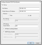
Configue Standard TCP/IP Port Monitor Screen
