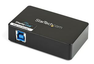
The USB32HDDVII USB 3.0 to HDMI and DVI-I Dual Head Adapter turns an available USB 3.0 port into one DVI-I or VGA port (DVI to VGA adapter included) and one HDMI output, with support for high-definition 1080p and 1920x1200 video and 5.1 surround sound audio (from HDMI port only). Each display can simultaneously support the maximum resolution of 2048x1152 @ 60Hz.
