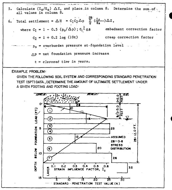
FIGURE 7 (continued) Settlement of Footings Over Granular Scils: Example Computation Using Schmertmann's Method
