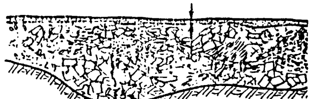
a. RUBBISH DUMP: UNCONTROLLED PLACEMENT, NO COMPACTION
