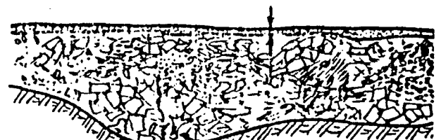
a. RUBBISH DUMP: UNCONTROLLED PLACEMENT, NO COMPACTION
