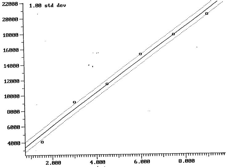
Calibration Plot (Ext Stds) Filename: T014GB Correlation Coeff: 0.994 Toluene Compound: 26 of 45 Standard Deviation: 1.547 (Peak Area of Sample) vs (Amount of Sample Injected) (LiniLin)
