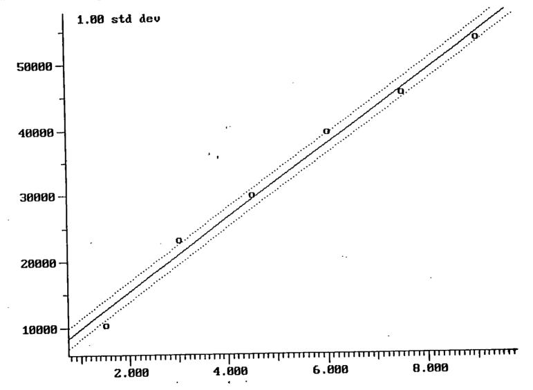
Calibration Plot (Ext Stds) Filename: T014GB Correlation Coeff: 0.996 1,2-Dibromoethane Compound: 27 of 45 Standard Deviation: 0.768 (Peak Area of Sample) vs (Amount of Sample Injected) (LiniLin)
