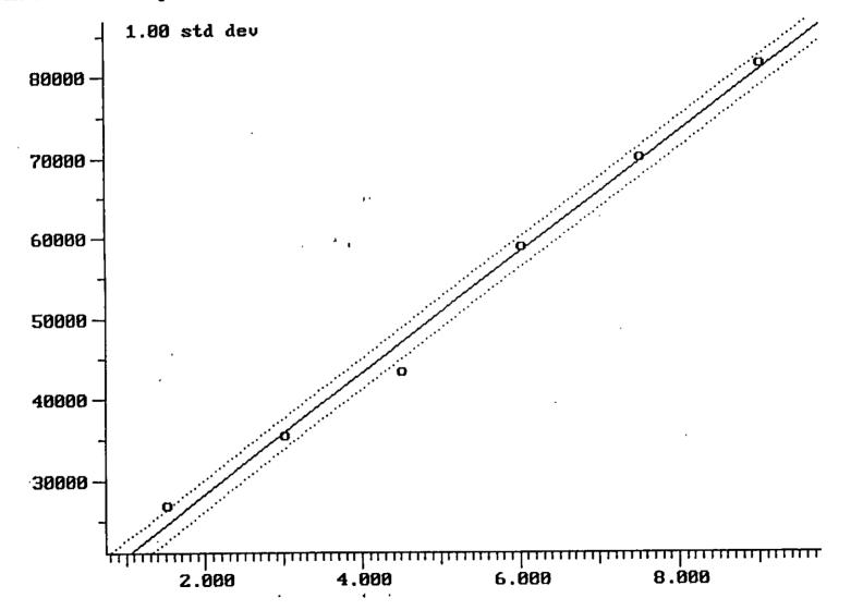
Calibration Plot (Ext Stds) Filename: T014GB Correlation Coeff: 0.992 1,3-Dichlorobenzene Compound: 40 of 45 Standard Deviation: 1.216 (Peak Area of Sample) vs (Amount of Sample Injected) (Lin!Lin)
