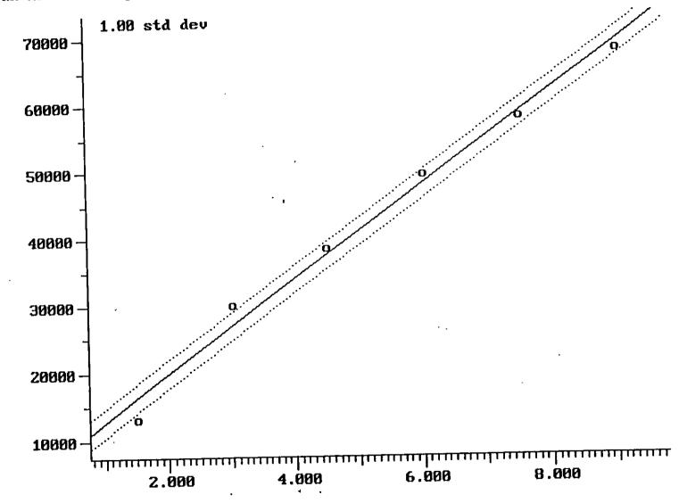
Calibration Plot (Ext Stds) Filename: T014GB Correlation Coeff: 0.993 Freon 113 Compound: 11 of 45 Standard Deviation: 0.783 (Peak Area of Sample) vs (Amount of Sample Injected) (LiniLin)
