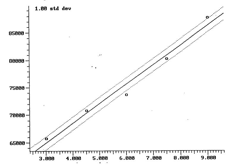
Calibration Plot (Ext Stds)Filename: T014GBCorrelationCoeff: 0.982HexachlorobutadieneCompound: 45 of 45Standard Deviation: 0.156(Peak Area of Sample) vs (Amount of Sample Injected)(Lin!Lin)
