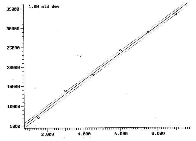
Calibration Plot (Ext Stds)Filename: T014GBCorrelationCoeff: 0.9984-BromofluorobenzeneCompound: 35 of 45Standard Deviation: 0.585(Peak Area of Sample) vs (Amount of Sample Injected)(Lin!Lin)
