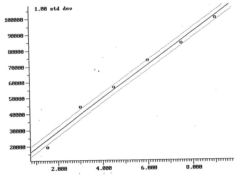
Calibration Plot (Ext Stds) Filename: T014GB Correlation Coeff: 0.993 Carbontetrachloride Compound: 20 of 45 Standard Deviation: 1.122 (Peak Area of Sample) vs (Amount of Sample Injected) (Lin!Lin)
