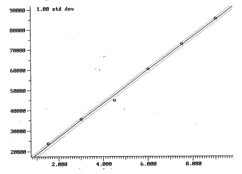
Calibration Plot (Ext Stds) Filename: T014GB Correlation Coeff: 0.997 1,3,5-Trimethylbenzene Compound: 38 of 45 Standard Deviation: 1.725 (Peak Area of Sample) vs (Amount of Sample Injected) (LiniLin)
