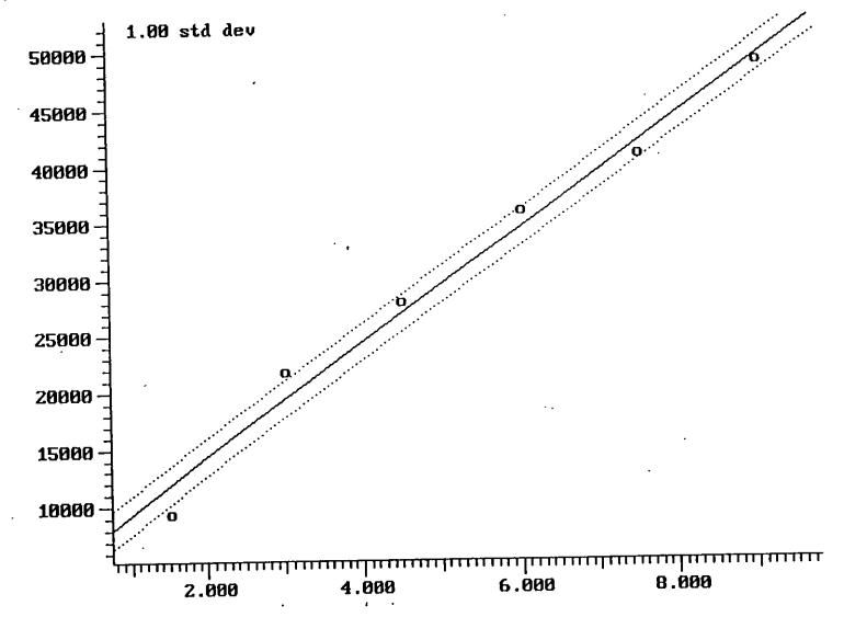
Calibration Plot (Ext Stds) Filename: T014GB Correlation Coeff: 0.992 Chloroform Compound: 16 of 45 Standard Deviation: 1.762 (Peak Area of Sample) vs (Amount of Sample Injected) (LiniLin)
