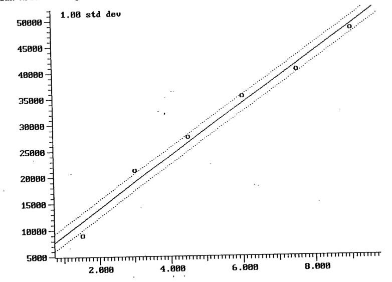
Correlation Coeff: 0.992 Filename: TO14GB Calibration Plot (Ext Stds) Standard Deviation: 1.622 Compound: 14 of 45 1,1-Dichloroethane (Lin!Lin) (Peak Area of Sample) vs (Amount of Sample Injected) 1.00 std dev 50000 45000 40000 35000 30000 25000 20000 15000 10000 8.000 6.000 4.000 2,000 ÷ .
