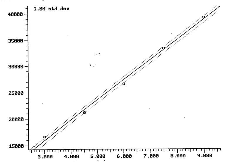
Calibration Plot (Ext Stds) Filename: T014GB Correlation Coeff: 0.986 1,2,4-Trichlorobenzene Compound: 43 of 45 Standard Deviation: 0.458 (Peak Area of Sample) vs (Amount of Sample Injected) (Lin!Lin)
