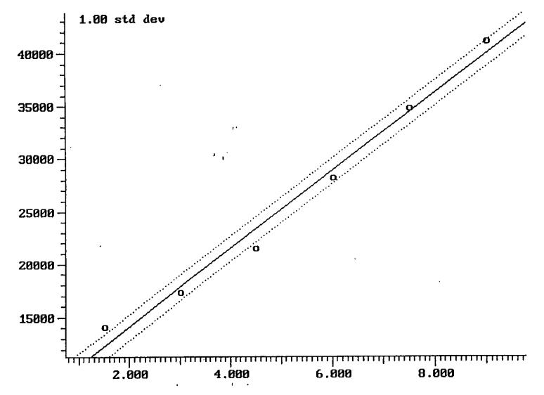
Calibration Plot (Ext Stds) Filename: T014GB Correlation Coeff: 0.997 Standard Deviation: 0.982 Compound: 41 of 45 1,4-Dichlorobenzene (LinlLin) (Peak Area of Sample) vs (Amount of Sample Injected)
