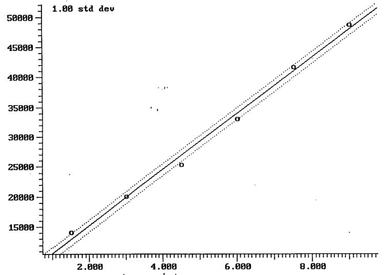
Calibration Plot (Ext Stds) Filename: T014GB Correlation Coeff: 0.998 1,2-Dichlorobenzene Compound: 42 of 45 Standard Deviation: 0.546 (Peak Area of Sample) vs (Amount of Sample Injected) (Lin!Lin)
