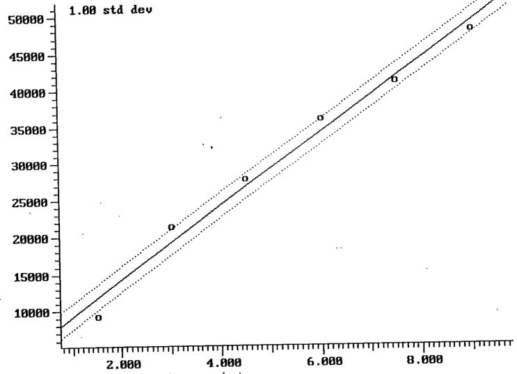
Calibration Plot (Ext Stds) Filename: T014GB Correlation Coeff: 0.988 1,1,1-Trichloroethane Compound: 18 of 45 Standard Deviation: 1.163 (Peak Area of Sample) vs (Amount of Sample Injected) (LiniLin)
