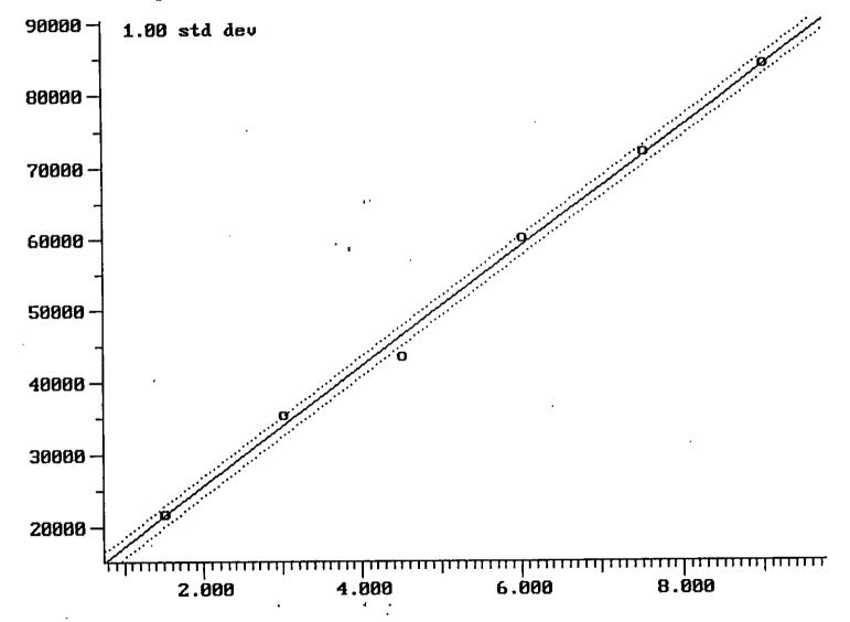
Calibration Plot (Ext Stds)Filename: T014GBCorrelationCoeff: 0.9984-EthyltolueneCompound: 37 of 45Standard Deviation: 1.225(Peak Area of Sample) vs (Amount of Sample Injected)(Lin:Lin)
