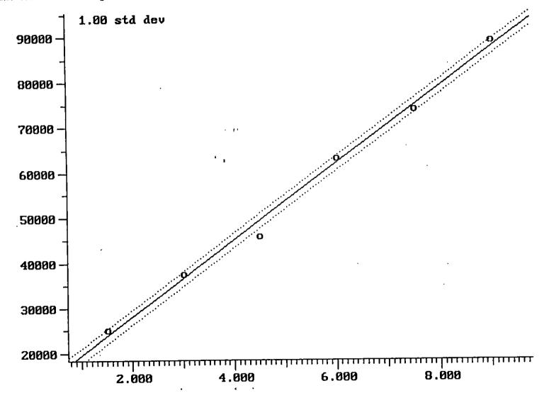
Calibration Plot (Ext Stds) Filename: T014GB Correlation Coeff: 0.995 1,2,4-Trimethylbenzene Compound: 39 of 45 Standard Deviation: 1.830 (Peak Area of Sample) vs (Amount of Sample Injected) (LiniLin)
