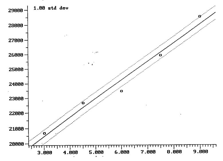
Calibration Plot (Ext Stds) Filename: T014GB Correlation Coeff: 0.987 Naphthalene Compound: 44 of 45 Standard Deviation: 1.213 (Peak Area of Sample) vs (Amount of Sample Injected) (Lin!Lin)
