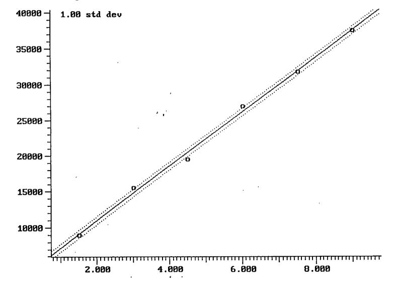
Calibration Plot (Ext Stds) Filename: T014GB Correlation Coeff: 0.998 Benzylchloride Compound: 36 of 45 Standard Deviation: 1.452 (Peak Area of Sample) vs (Amount of Sample Injected) (Lin!Lin)
