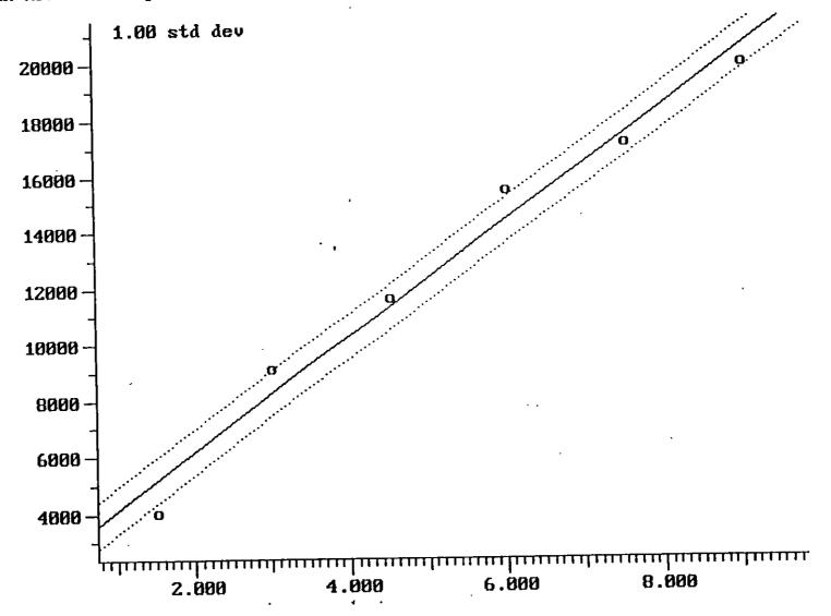
Calibration Plot (Ext Stds) Filename: T014GB Correlation Coeff: 0.992 Trichloroethene Compound: 22 of 45 Standard Deviation: 0.863 (Peak Area of Sample) vs (Amount of Sample Injected) (Lin!Lin)
