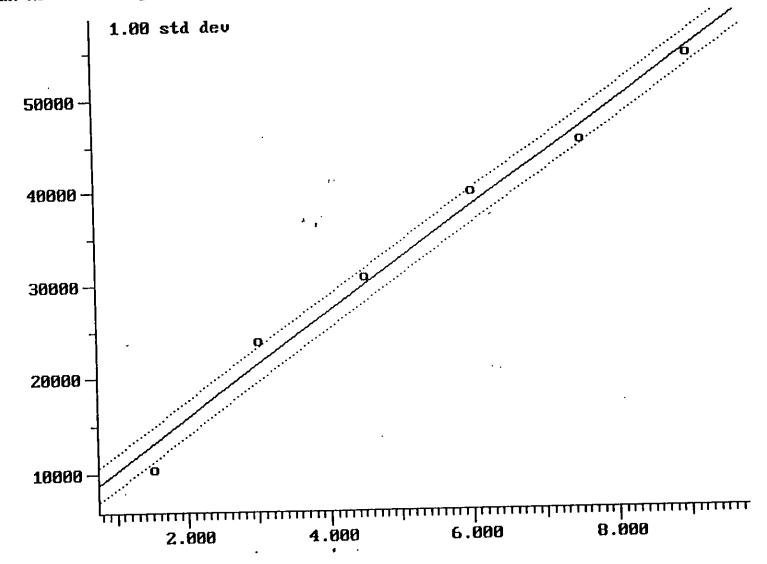
Correlation Coeff: 0.992 Filename: T014GB Calibration Plot (Ext Stds) Standard Deviation: 1.675 Compound: 17 of 45 1,2-Dichloroethane (Lin¦Lin) (Peak Area of Sample) vs (Amount of Sample Injected)
