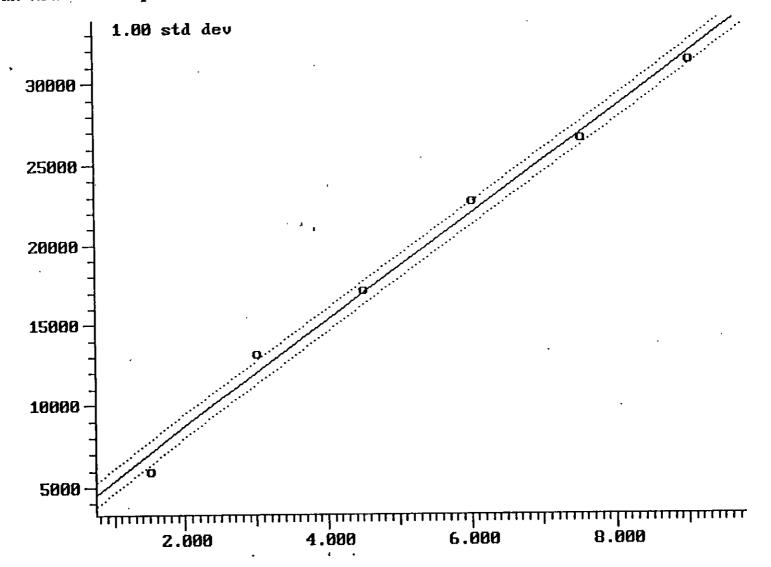
Calibration Plot (Ext Stds) Filename: T014GB Correlation Coeff: 0.993 Tetrachloroethene Compound: 28 of 45 Standard Deviation: 0.342 (Peak Area of Sample) vs (Amount of Sample Injected) (LiniLin)
