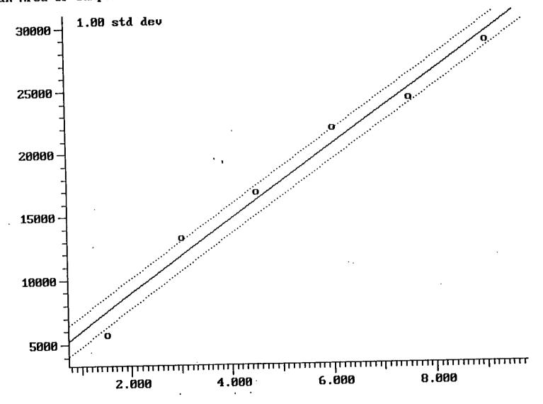
Calibration Plot (Ext Stds) Filename: T014GB Correlation Coeff: 0.993 Benzene Compound: 19 of 45 Standard Deviation: 3.199 (Peak Area of Sample) vs (Amount of Sample Injected) (LiniLin)
