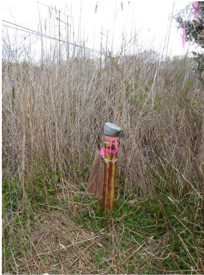
Groundwater monitoring well ERM-101S
