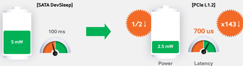
Figure 12. Power management of the 950 PRO using L1.2
