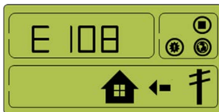
[Figure 4-19: Event occurrence, PV string2 over current protection]
