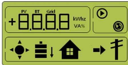
[Figure 4-2: PV generation, battery charge, Load use, sell remaining amount]
