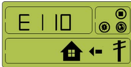
[Figure 4-21: Event occurrence, Battery over current protection]
