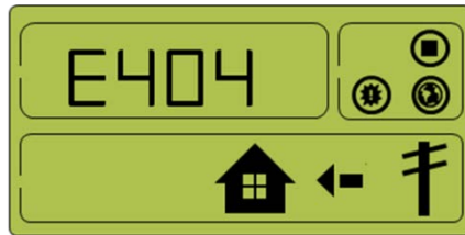
[Figure 4-31: Event occurrence, PV mis-wiring]
