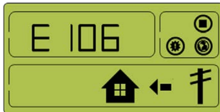
[Figure 4-17: Event occurrence, PV string1 over current protection]
