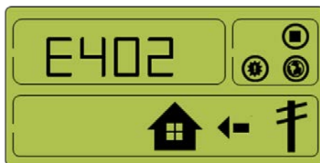
[Figure 4-29: Event occurrence, Over Current TZ Fault]
