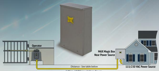
2-Wires, 24VDC Low Voltage Power
