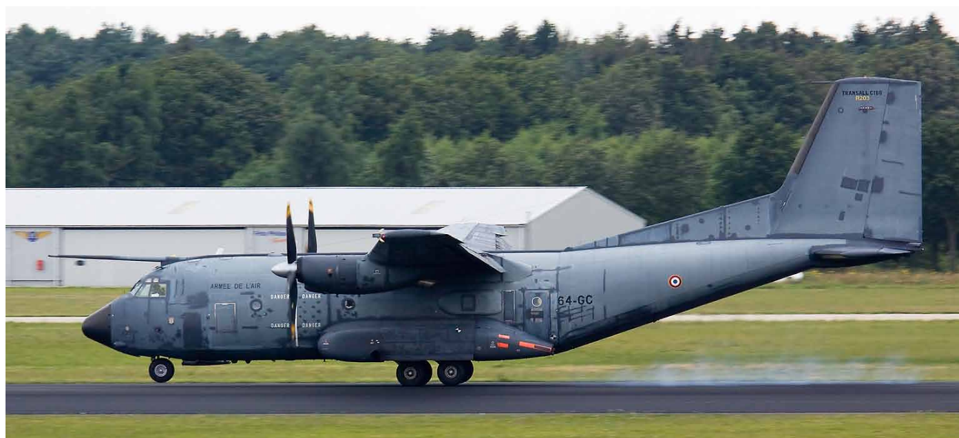
Seen here on the runway at Eindhoven is C-160R R203/64-GC of ET00.064. It differs from the regular C-160R in that it is also an airborne tanker aircraft. The tankers can be identified by the dayglo applied to the rear of the fairing covering the main undercarriage. It was at Eindhoven for a change of command with the EATC. (24 July 2012, Mike Schoenmaker)
