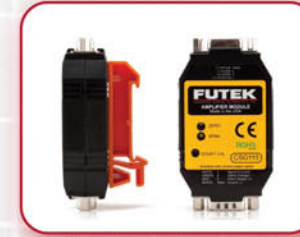
CSG110 , Strain Gage Amplifier , Standard , Enclosed With Din Rail Mount , With DB9 Connectors , ABS-94HB Black Enclosure , Analog Output , +/-5 VDC , +/-10 VDC , 0-20 mA , 4-20 mA , 0-16 mA , 5-25 mA , 1 KHZ Bandwidth & up to 25 KHZ
