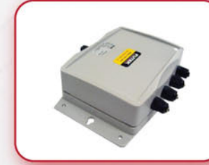
IAC200 , Junction Box - 4 Channel , Nema 4 Rating , Material - Polyurethane , Analog Output , +/-5 VDC , +/-10 VDC , 0-20 mA , 4-20 mA , 0-16 mA , 5-25 mA
