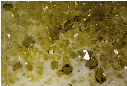
Figure 1. Crystals of \text{Ce}_2\text{Sn}_2\text{O}_7 (1-2mm)
