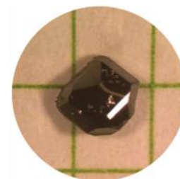
Figure 5. Optical microscope image of the grown crystals. Background is mm-sized grid.
