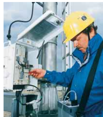
The Level Meter R&S® URV35 with the Insertion Unit R&S® URV5-Z2 in mobile use
