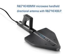
The R&S®HE400MW antenna handle operates from 20 MHz to 20 GHz. It supports the R&S<sup>®</sup>HE400VHF, R&S<sup>®</sup>HE400UWB, R&S<sup>®</sup>HE400LP, R&S®HE400CEL, R&S®HE400SCB and R&S®HE400SHF antenna modules and is compatible with the R&S®Spectrum Rider FPH handheld spectrum analyzer (models .13/.23/.26/.36), the R&S®FSH13 and R&S®FSH20 handheld spectrum analyzers and the R&S®Cable Rider ZPH cable and antenna analyzer (model .12).
