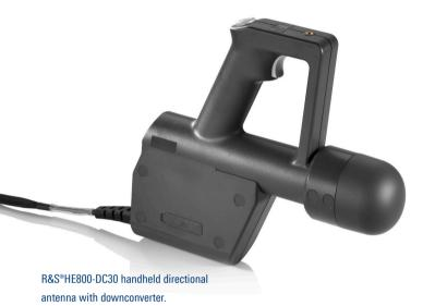
The antenna consists of an antenna handle with an integrated downconverter, a fixed antenna module behind the foam radome and an RF and supply cable to the receiver.
