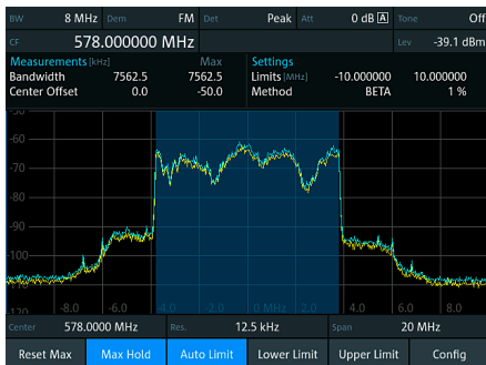
Automatic occupied bandwidth measurement of a DVB-T signal ( \beta % method).
