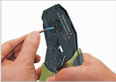
Insert ferruled conductor into crimping station.
