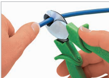
Cutting a conductor.
