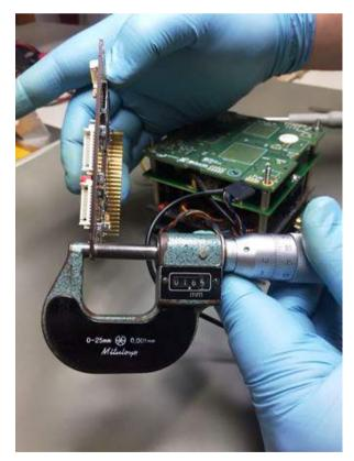
Figure 3 – Electrical Engineering student at LITN using a micrometer to evaluate the thickness of a PCB.
