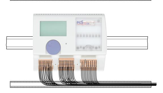
On the PCS1 the terminals are accessible without removing the cover.
