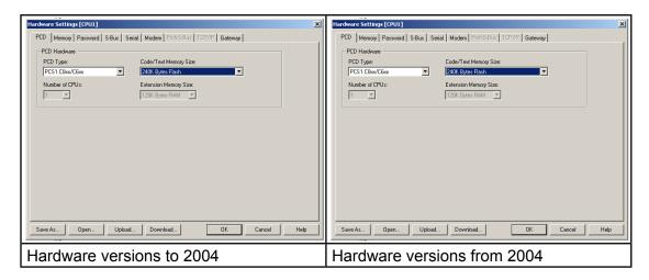
There are only 128 kB of flash EPROM available for code/text memory. One block of memory is lost to configuration data (header), because flash EPROM can only be accessed in block mode.
