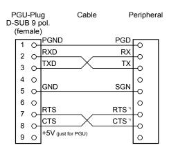
1) When communicating with terminals, check whether some connections are provided with bridges or need to be set to "H" or "L" with the "SOCL" instruction. It is generally recommended to use a handshake (RTS/CTS).
