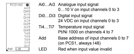
The FBox converts the signals into the input channels for the PCS1. The first 4 inputs can be used as analogue 0...10 VDC or digital 24 VDC inputs. The last 4 inputs are interpreted as Pt/Ni 1000 for temperature values. The sensor type is selected in the FBox. The error output displays which input is showing an error caused by invalid values (bit 0 for input 0, bit 1 for input 1 etc.). This allows e.g. a sensor fault to be detected. Resolution of analogue signals: 10 bit (0.6 °C).
