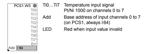
The FBox converts the signals to the input channels on the PCS1 with a resolution of 12 bits (max. 0.15 °C for Pt 1000, max. 0.08 °C for Ni 1000). All inputs are interpreted as Pt/Ni 1000. The sensor type can be selected in the FBox. The error output displays which input is showing an error caused by invalid values (bit 0 for input 0, bit 1 for input 1 etc.). This allows e.g. a sensor fault to be detected.
