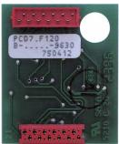
**PCD7.F120:**RS-232 with RTS/CTS, DTR/DSR, DCD, suitable for modem connection, for Slot A
