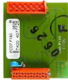
PCD7.F180: Connecting module for MP-Bus, for Slot A
