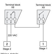
Wiring details Example of a 2-stage fan controller with mutual latching
