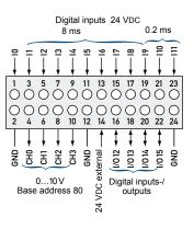
If combined I/Os 12...15 are used as outputs, an external supply is required (24 VDC external). In such cases only source operation will be possible at the inputs.
