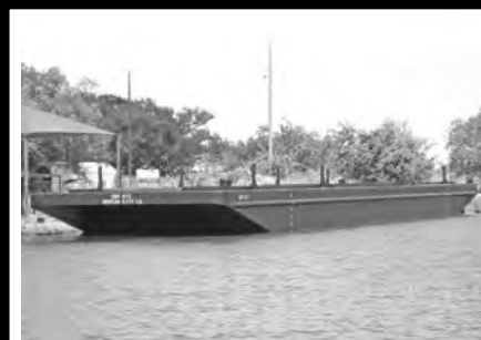
DECK BARGES 120'0" x 30' 0" x 7'0" Double or Single Rake
