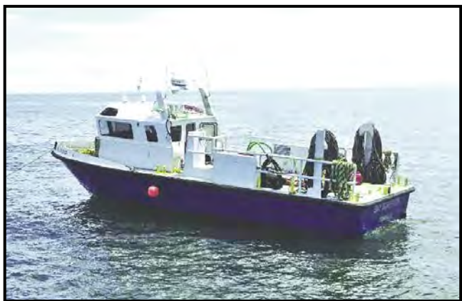
BAY SURVEYOR — CREW BOAT 45'x15'x3.5' CONVERTED TO ACCOMADATE DIVE CREWS AND SURVEY EQUIPMENT
