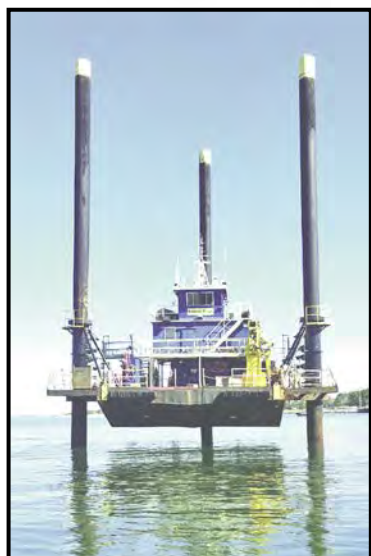
LIFT BOAT "CAPT RAY" 64'x32'x7' THRU-DECK DRILL WELL 70' — 15 TON DECK CRANE 8-71 DETROITS 13,000 GAL FUEL CAPACITY BERTHING FOR 8 GALLEY 450 GAL FRESH WATER TANK 35 GPH FRESH WATER MAKER
