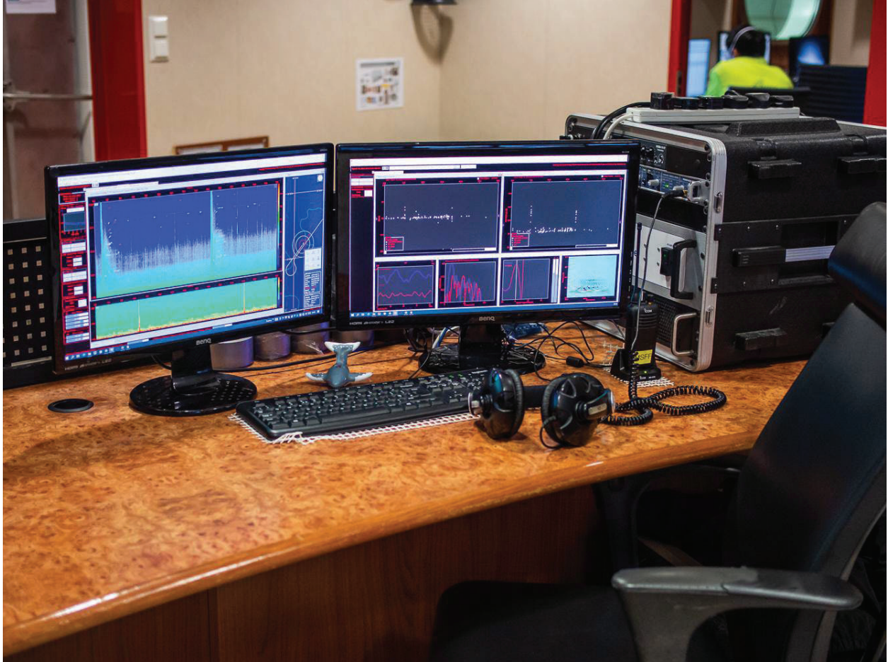
Figure 11: Passive acoustic monitoring station in instrument room.
