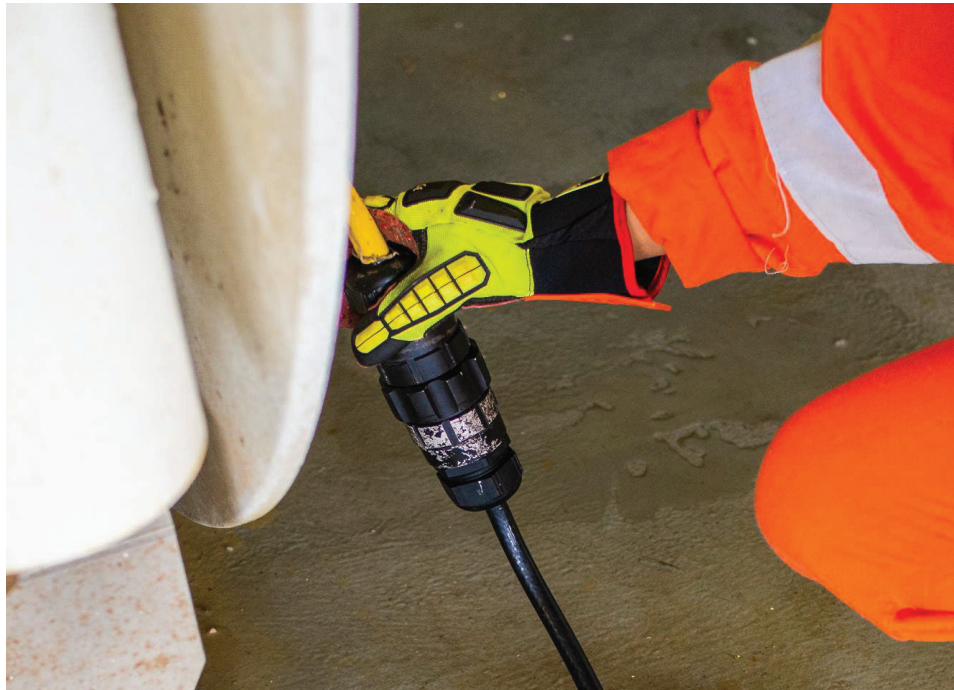
Figure 5. Connection between tow cable and deck cable located on winch.
