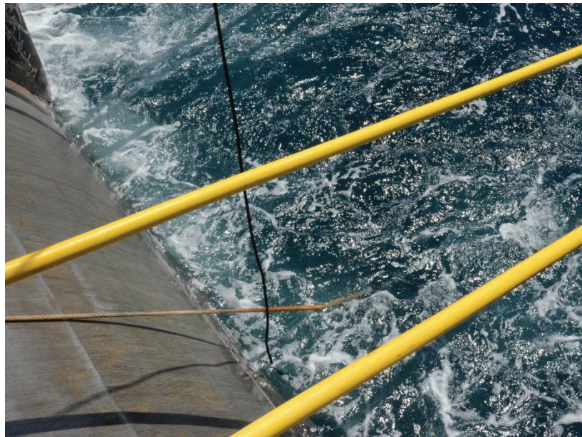
Figure 9. When deployed the cable is completely submerged at 100 meters and underneath umbilicals
