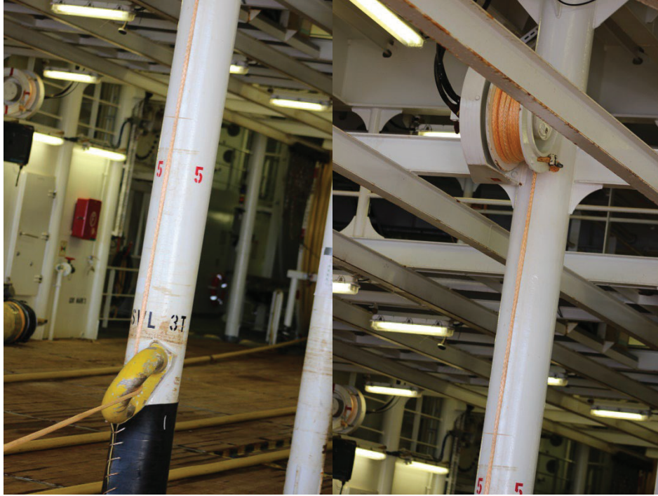
Figure 8. Rope from gun deck winch that attaches to Chinese finger
