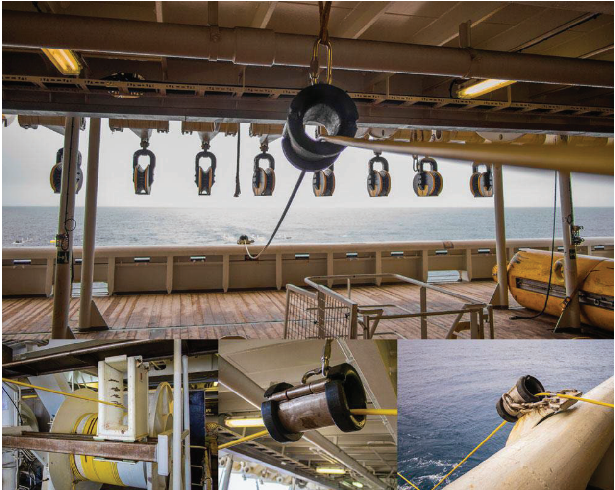
Figure 2. Deployed of tow cable showing directionality, position on winch, sliding collar from ceiling, and sliding collar at the ships stern.
