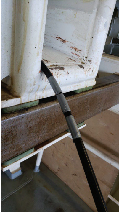
Figure 10 . PAM cable marked at winch; excess cable taped on streamer deck
