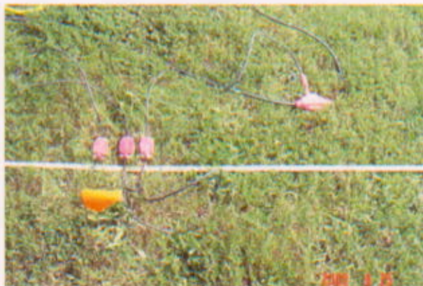
Figure 18. A three-geophone array was used at each takeout
