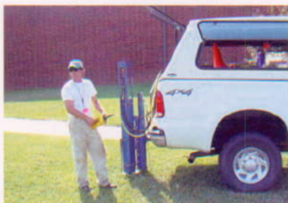
Figure 20. Truck mounted spring actuated hammer seismic energy source
