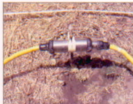
Figure 10. SuperSting electrode attached to stake
