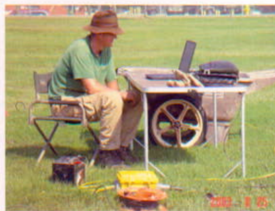
Figure 21. PC controlled refraction data collection
