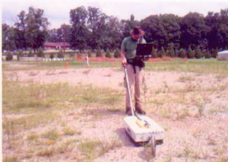
Figure 36. GPR data acquisition, 250 MHz antenna
