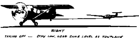
TAKING OFF — STAY LOW, NEAR SAME LEVEL AS TONPLANE —Joy of Soaring
