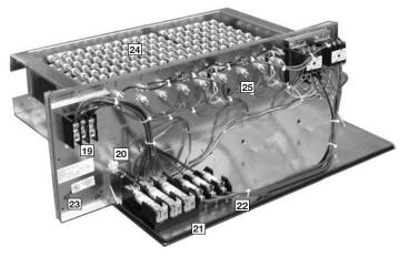
Power hook-up in the field is easy with single-point wiring to a terminal block (19) and a polarized plug for the low-voltage connection (20). The electric furnace comes with fuses for the unit (21) and for the electric furnace (22), and is UL certified (23). The electric heating elements are of a wound-wire construction (24) and isolated with ceramic bushings. The limit switch (25) protects the design from over-temperature conditions.
