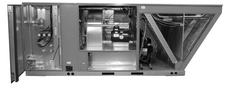
Inside the control box (1), each electrical component is clearly identified with a label that matches the component to the wire diagram for ease of trouble shooting. All wiring is numbered on each end of the termination and color-coded to match the wiring diagram. The control transformer has a low voltage circuit breaker that trips if a low voltage electrical short occurs. There is a blower contactor and contactor for each compressor.
