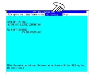
3) Select the [data Transmission] command. After pushing [Alt] at once, select it with the →key or the [T]key. Appear the screen for selecting the transmitting direction of data by pushing Select Read (Model E →Personal computer) with the [Enter][↓] key, after that pushing [Enter].
