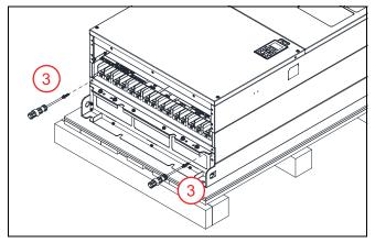
Install the conduit box to the drive using the following screws and nuts tightened to a torque of: M6 Screws 1 - 6: 55-65 kg-cm / 47.7-56.4 lb-in / 5.4-6.4 Nm
