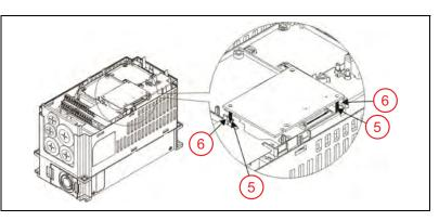
When clips are secure, install retaining screws and tighten to a torque of 6-8 kg-cm / 5.2-7 lb-in. / .59-.79 Nm.
