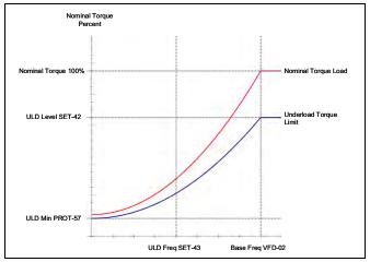
for Underload or No-Flow conditions, which protects against nuisance faults. The delay operates at any VFD start, in both Hand and Auto modes, including Run, Wake, Restart, or Reset commands.
