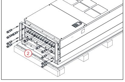
3. Fasten the M6 screws to two locations. Tighten screws to a torque of 35-45 kg-cm / 30.3-39 lb-in. / 3.4-4.4 Nm.
