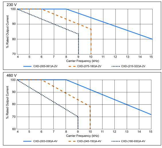
230 V / 460 V Permanent Magnet Motor with SVC Control
