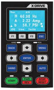
Hand Run Command [SET-10]: Source of Run Command in Hand mode. VFD starts based on input from:
