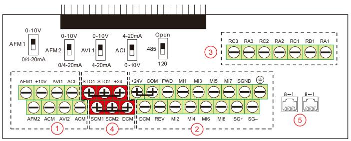
The control board is divided into 5 groups of terminals and connectors, plus a group of micro switches that control individual terminal configurations.
