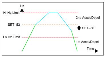
**Second ACC [SET–54]:** Time in seconds for drive to accelerate from 0 Hz to maximum frequency. This rate takes effect when frequency is above [SET–53]. Default = 60 sec.
