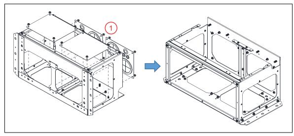
2. Remove the screws shown from the bottom of the drive and remove the bracket.
