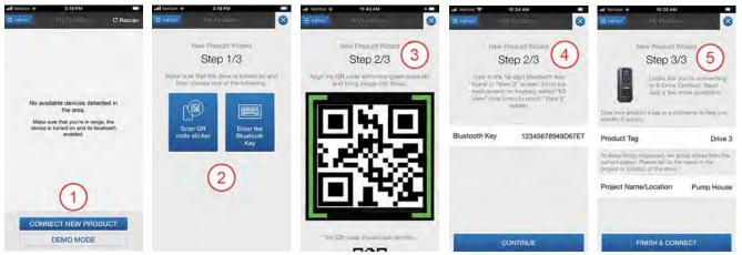
After installing the X-Drive Connect app on your device, use the following procedure to connect to a X-Drive:
