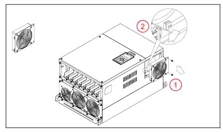
Frame E models use multiple heat sink fan styles. Be sure to order the correct part when replacing the fan.
