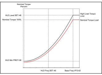
To enable High Load Detection, adjust the following parameters:
