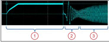
Advance V/F Control – With the motor started, frequency compensation stabilizes the current load. Torque compensation adjusts output voltage to correct for torque control.
