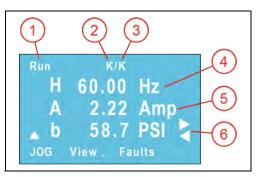
4. User Selectable Display Line 1. Use Arrow and Enter keys to step through selections and to change setpoints.
