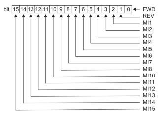
**View Screen 4:** This screen displays the status of the multi-function (digital) outputs in hex format. Solid boxes indicate that the output is active.
