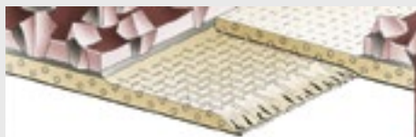
Overlapped joint with grit sanding
