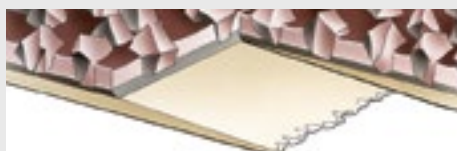
Overlapped joint without grit sanding
