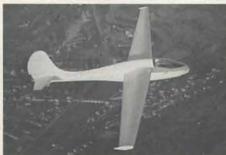
Fig 30. The Breguet 901 which was one of the first gliders to have flaps, a retractable undercarriage and the ability to carry waterballast (75kg).
