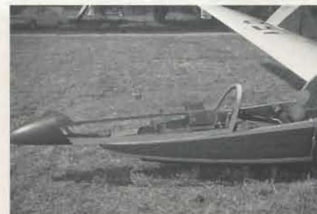
Fig 32. The cockpit of the Polish Standard Class Foka with its supine pilot seating.
