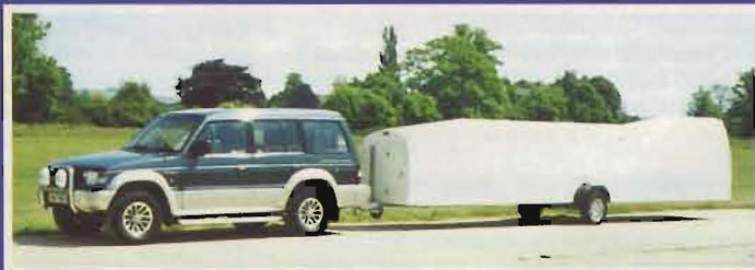
DF-15. Jig built aluminium trailer. Fully galvanised chassis. Acrylic coated super gloss white finish.
