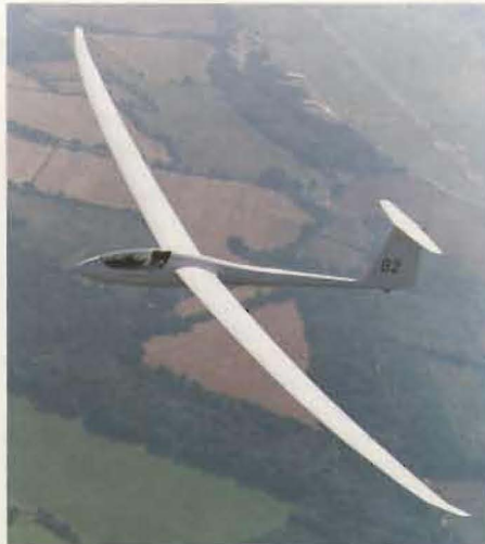
Fig 41. The 26.4m Nimbus 4 was designed by Klaus Holighaus - the ultimate performance production single-seater with an aspect ratio of 38.7 and L/D of 60. Photo: Julian Herbert.
