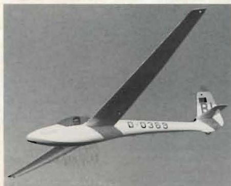
Fig 34. The Glasflügel Std Libelle of 1967 became very popular in its day, having good pilot view, retractable landing gear and pleasant handling characteristics.
