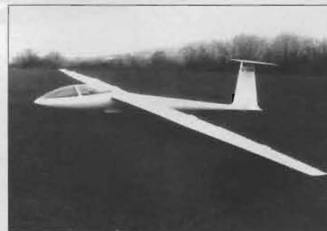
The D-36 Circe pioneered trailing-edge flaps
