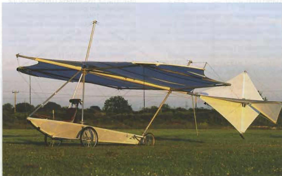
The 2003 replica of Sir George Cayley's 1853 man-carrying glider
