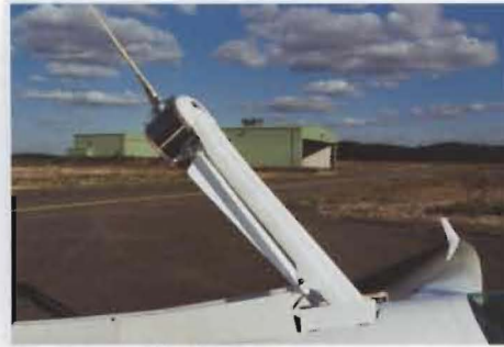
The pylon is travelling towards the upright position
