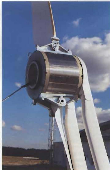
Main picture: Antares in flight. Above: propeller blades are mounted on the DC/DC brushless rotating engine
