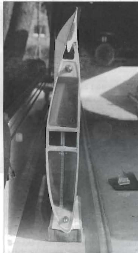
The outer join of the inner wing section of the ASW 28-18 prototype, with spring-loaded bolt and the connection tongue at the aileron (All photos: Jochen Ewald)
