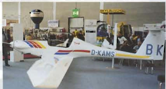
Above and below: the the Carat D-KAMS "BK" from AMS flight of Slovenia, with its unusual two-bladed propeller (seen here at rest) and its 15-metre "Discus" wings. The engine is a Sauer S1800-1-ES and the best glide, engine off, is claimed to be 35:1
