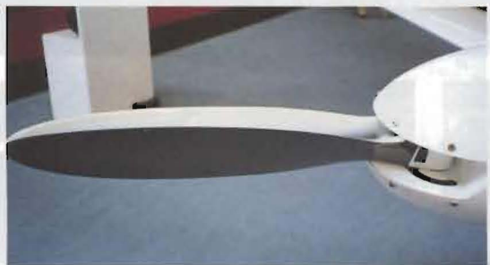
Above and below: the the Carat D-KAMS "BK" from AMS flight of Slovenia, with its unusual two-bladed propeller (seen here at rest) and its 15-metre "Discus" wings. The engine is a Sauer S1800-1-ES and the best glide, engine off, is claimed to be 35:1
