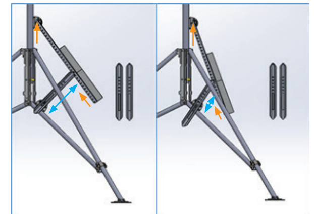
Figure 10: 50 degree to 70 degree mounting angles.
