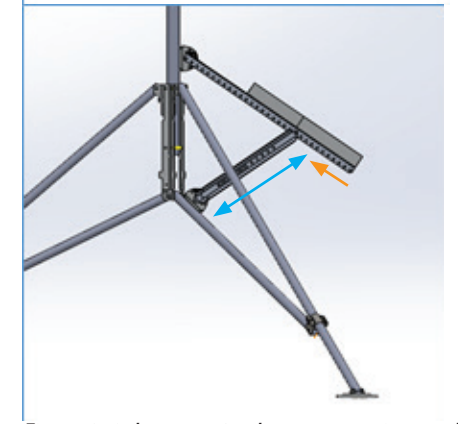
Figure 8: 0 degree to 35 degree mounting angles.
