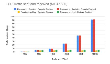
Figure 6: TCP traffic sent and received with a MTU of 1500. When Suricata is running, it runs in IDS mode alongside OvS and is only alerting.
