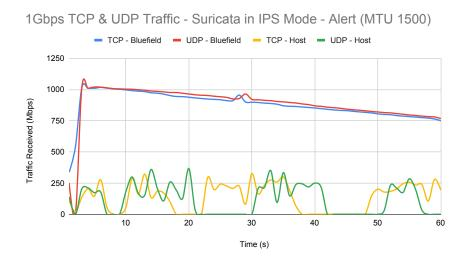
Figure 12: TCP and UDP traffic with a MTU of 1500 received on the BlueField and host. Suricata is running in IPS mode and is only alerting.
