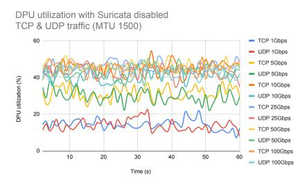
Figure 8: DPU utilization when Suricata is disabled and OvS enabled. Sending TCP & UDP traffic with a MTU of 1500.
