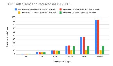
Figure 7: TCP traffic sent and received with a MTU of 9000. When Suricata is running, it runs in IDS mode alongside OvS and is only alerting.
