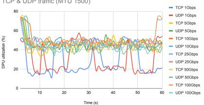
DPU utilization with Suricata enabled in IDS mode - Alert TCP & UDP traffic (MTU 1500)
