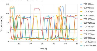
DPU utilization with Suricata enabled in IPS mode - Alert TCP & UDP traffic (MTU 1500)
