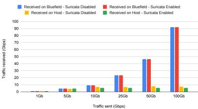
Figure 4: UDP traffic sent and received with a MTU of 1500. When Suricata is running, it runs in IDS mode alongside OvS and is only alerting.
