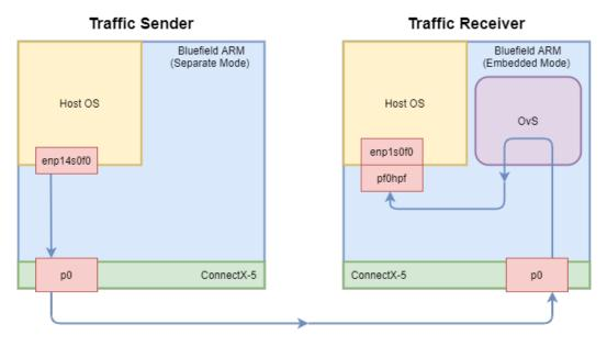
Figure 2: Overview of the basic experimental setup
