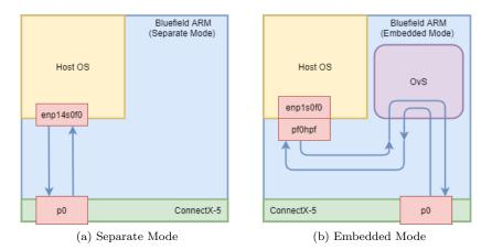
Figure 1: The two modes of operation on the BlueField
