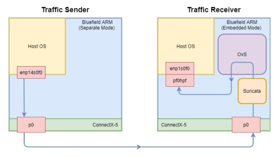
Figure 3: Overview of the experimental setup with Suricata installed on the receiving DPU in embedded mode
