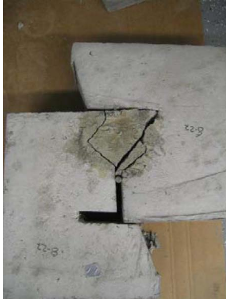
Figure 2.13 Shear Cracks at Failure (Porter 2009)
