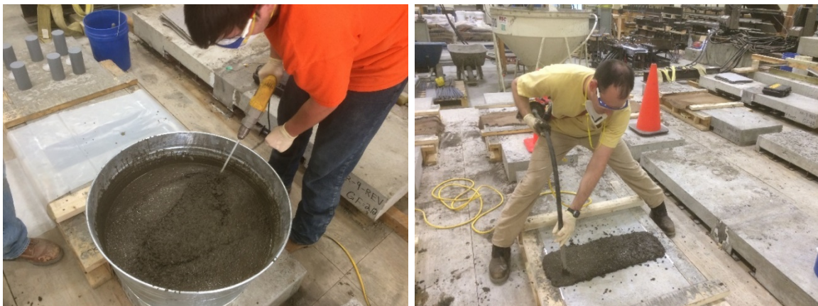
Figure 4.29 Mixing and Vibrating the Grout
