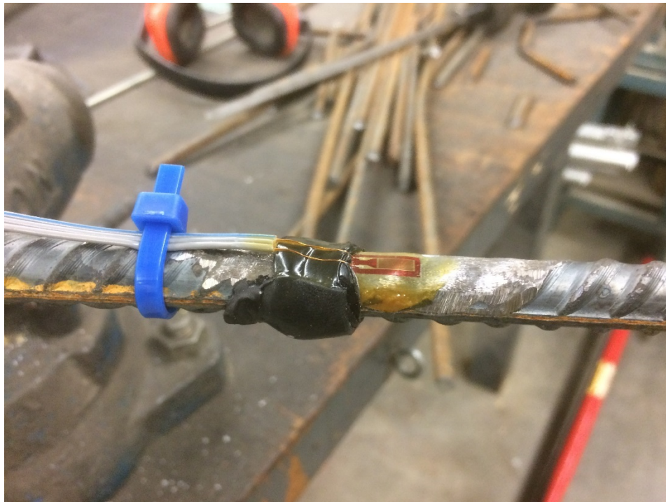
Figure 4.25 Electrical-Resistance Strain Gage (ERSG)
