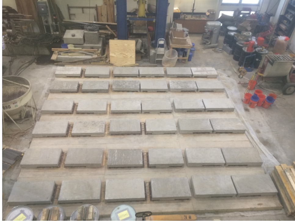
Figure 4.23 Overview of Panels before Grout Pour
