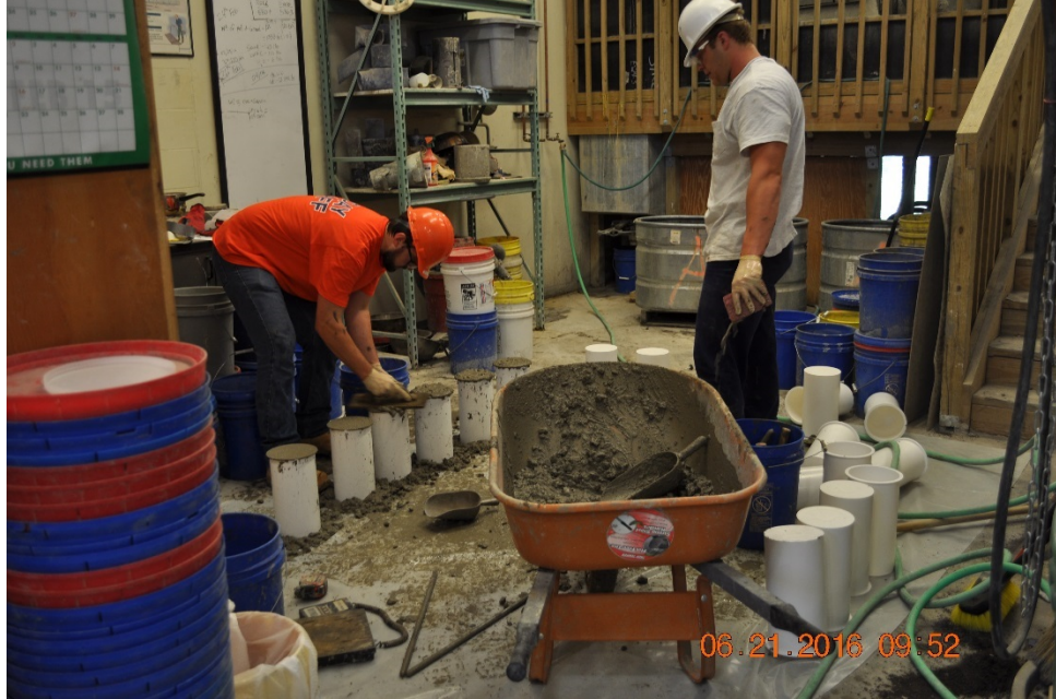
Figure 4.20 Material Testing of Deck Concrete
