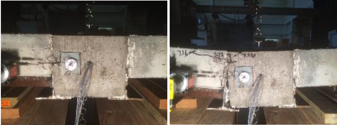
Figure 5.4 R-POS-Q Joint Before and After Test
