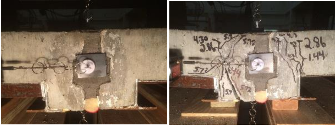
Figure 5.1 U-POS-Q Joint Before and After Test
