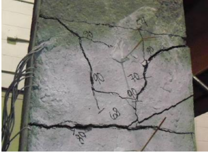
Figure 2.11 Tensile Cracks at Failure (Chapman 2010)
