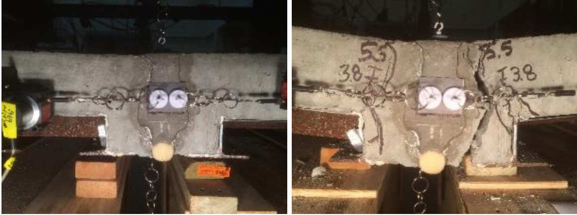
Figure 5.17 U-REV-Q Joint Before and After Test
