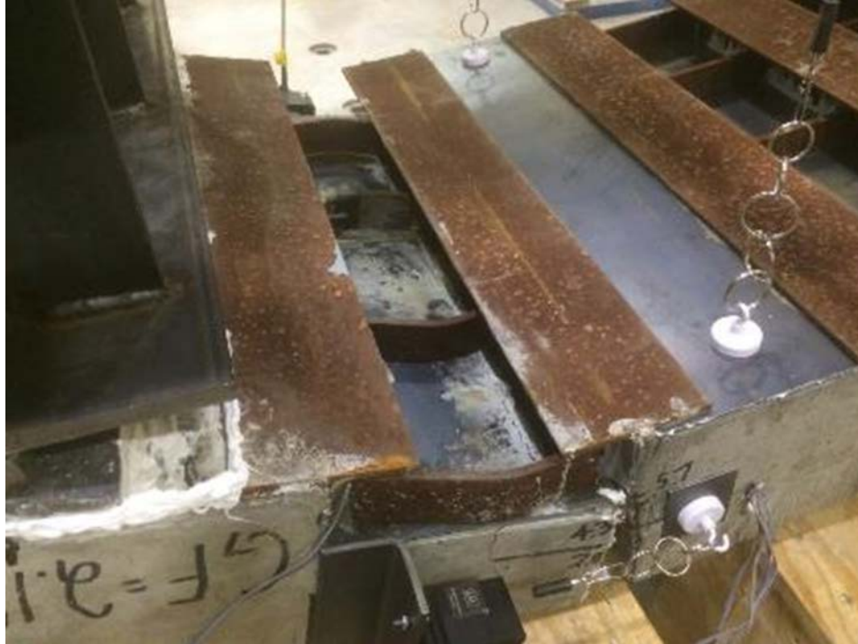
Figure 5.12 R-NEG-Q Buckled Distribution Bars (Inverted Specimen)
