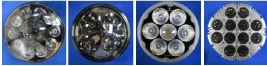
Figure 1: LED Samples Supplied by J.W. Speaker, Hydra-Tech International, Railhead/Divvali, and Smart Light Source Co. (Left to Right)
