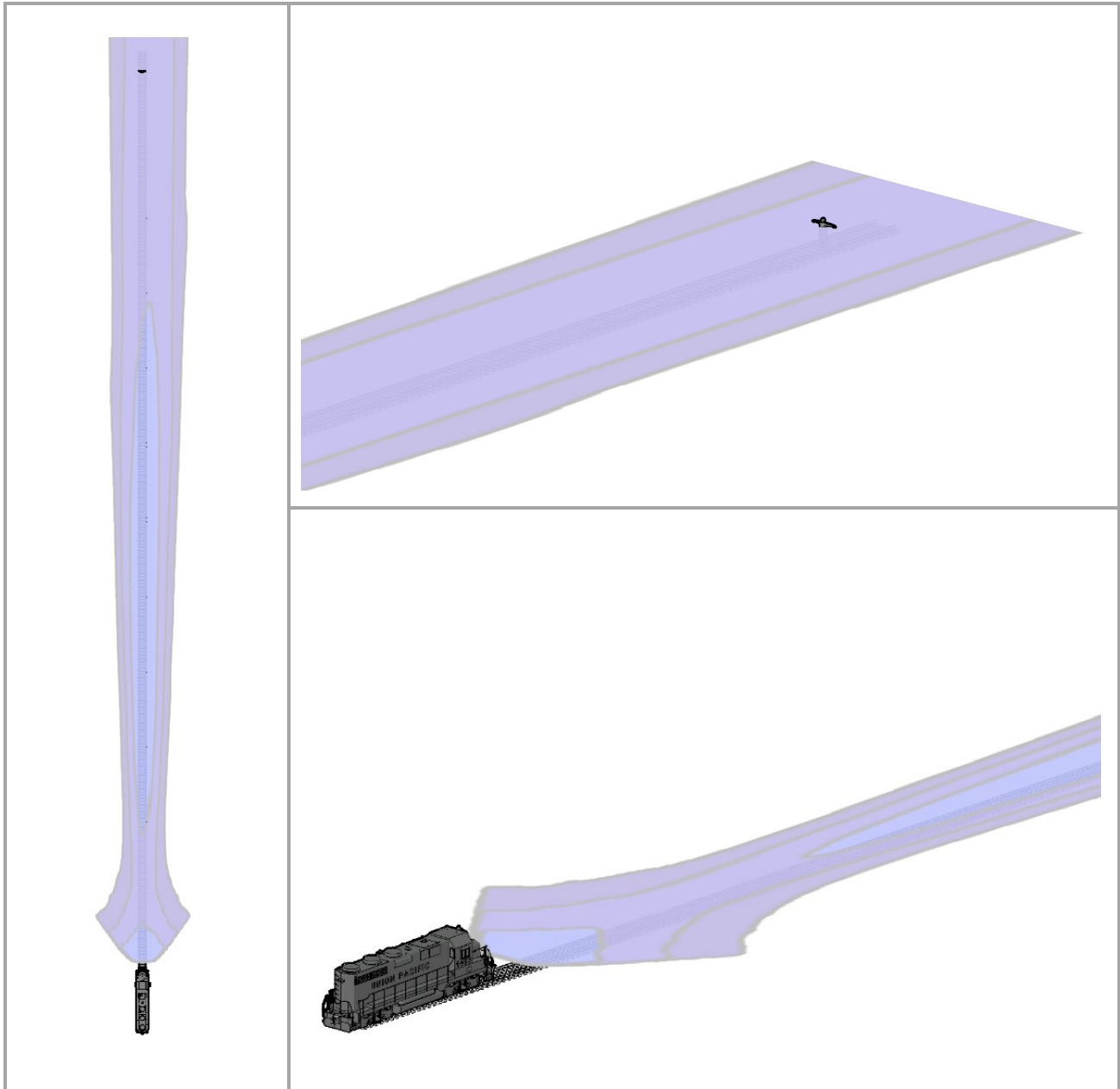
Figure 2. 3-Way View of an Illuminance map for a Hydra-Tech 2800K dual-lamp headlight (S5 LED). The human figure (upper-right plot) stands 800 ft away from the light source.
