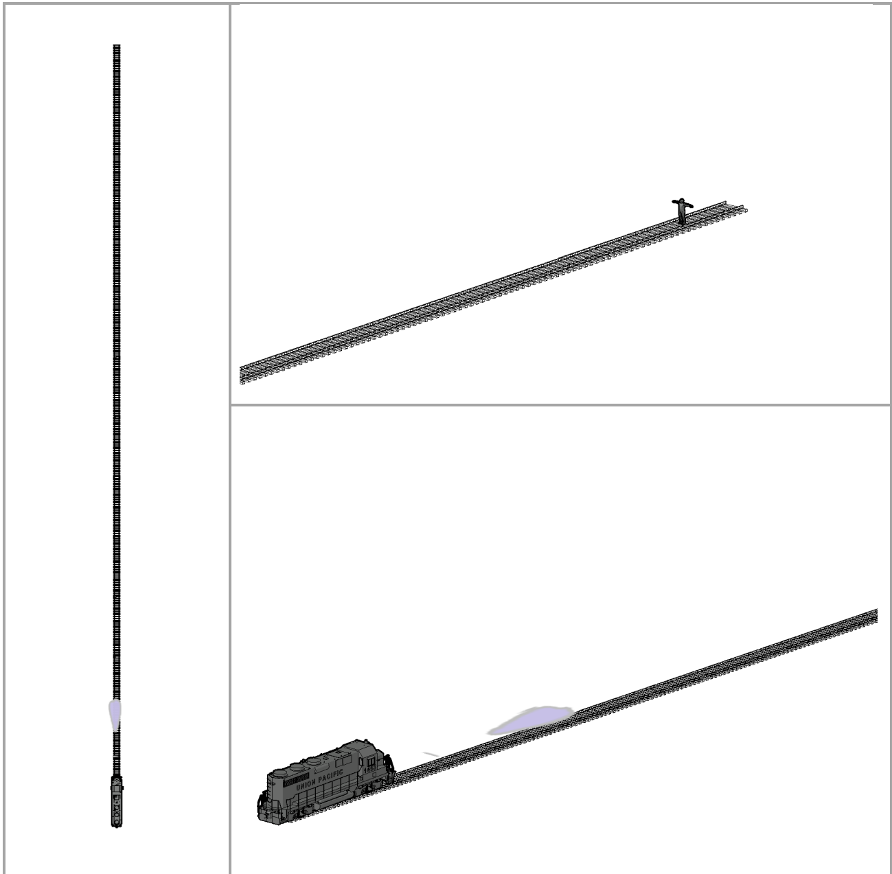
Figure 1. 3-Way View of an Illuminance map for a J.W. Speaker dual-lamp headlight (S2 LED). The human figure (upper-right plot) stands 800 ft away from the light source.
