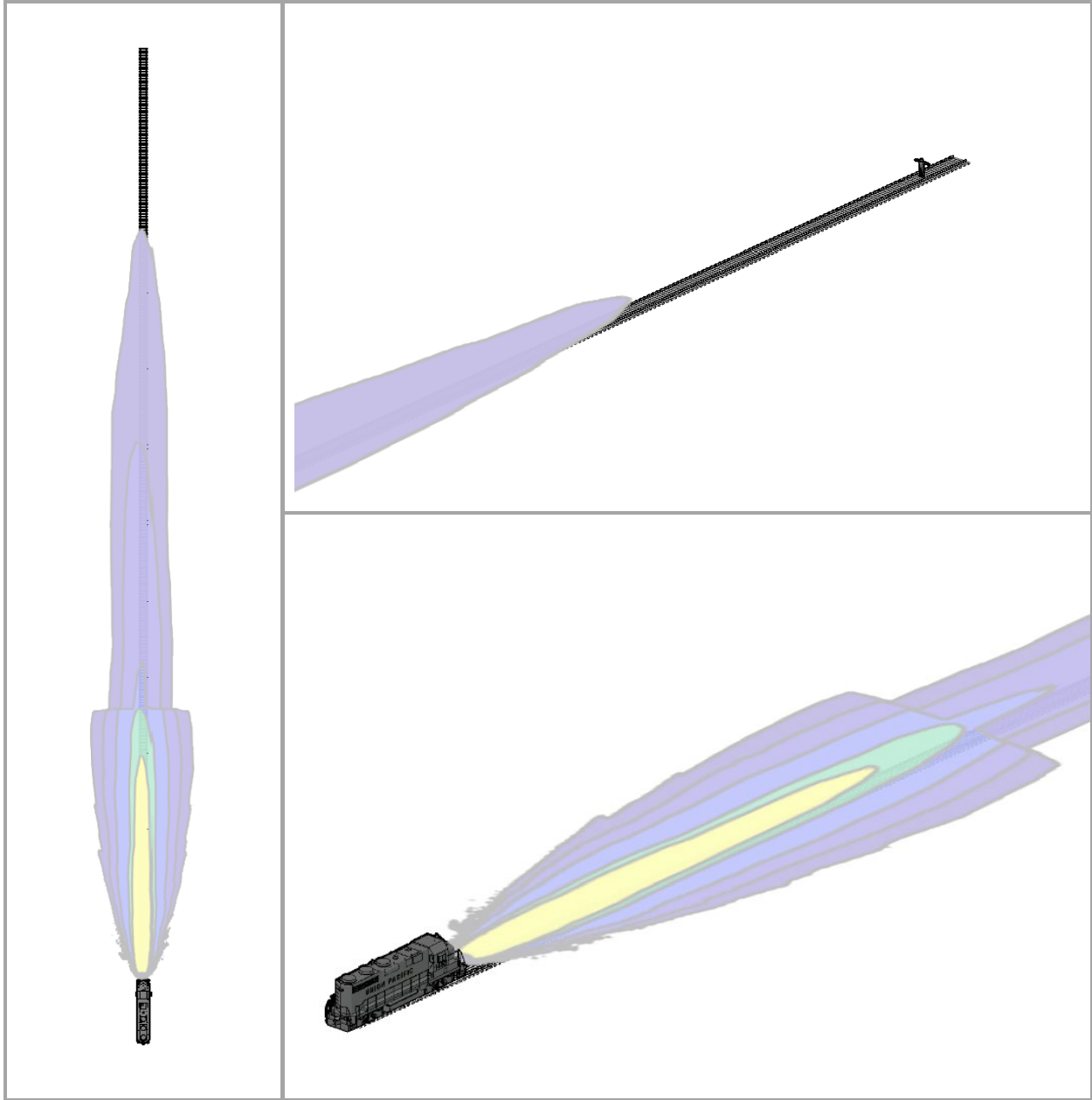
Figure 5. 3-Way View of an Illuminance map for a Smart Light Source dual-lamp headlight and auxillary lights (S3 LED). The human figure (upper-right plot) stands 800 ft away from the light source.
