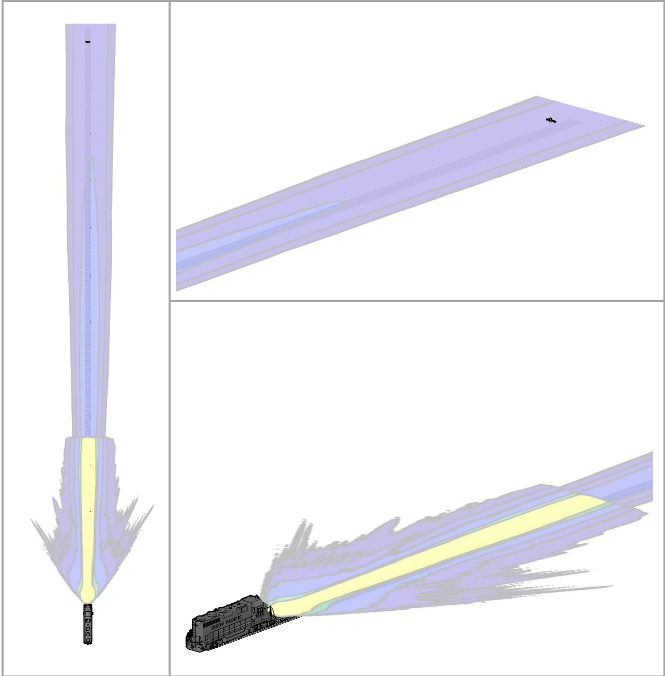
Figure 2. 3-Way View of an Illuminance map for a Hydra-Tech 2800K dual-lamp headlight and auxillary lights (S5 LED). The human figure (upper-right plot) stands 800 ft away from the light source.
