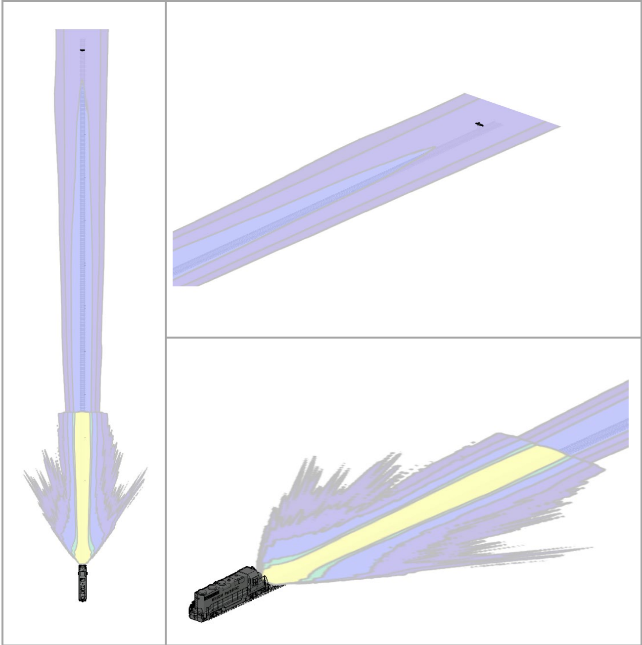
Figure 3. 3-Way View of an Illuminance map for a Hydra-Tech 7000K dual-lamp headlight and auxillary lights (S1 LED). The human figure (upper-right plot) stands 800 ft away from the light source.
