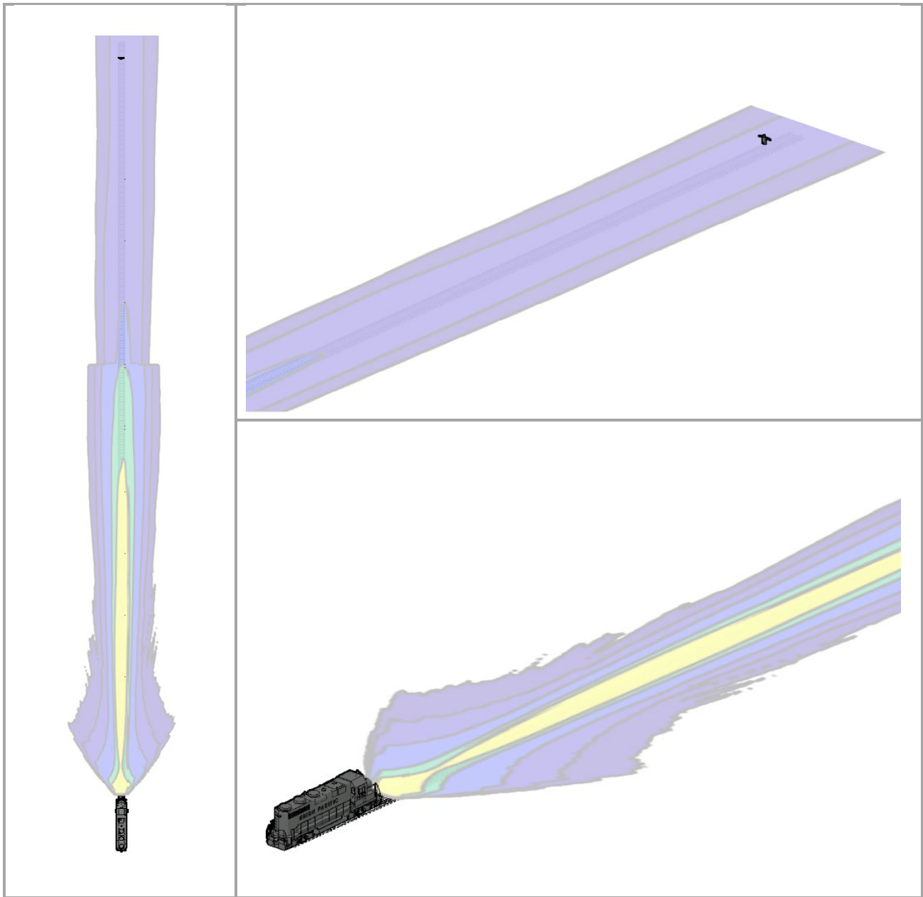
Figure 2. 3-Way View of an Illuminance map for a Hydra-Tech 2800K dual-lamp headlight and auxillary lights (S5 LED). The human figure (upper-right plot) stands 800 ft away from the light source.
