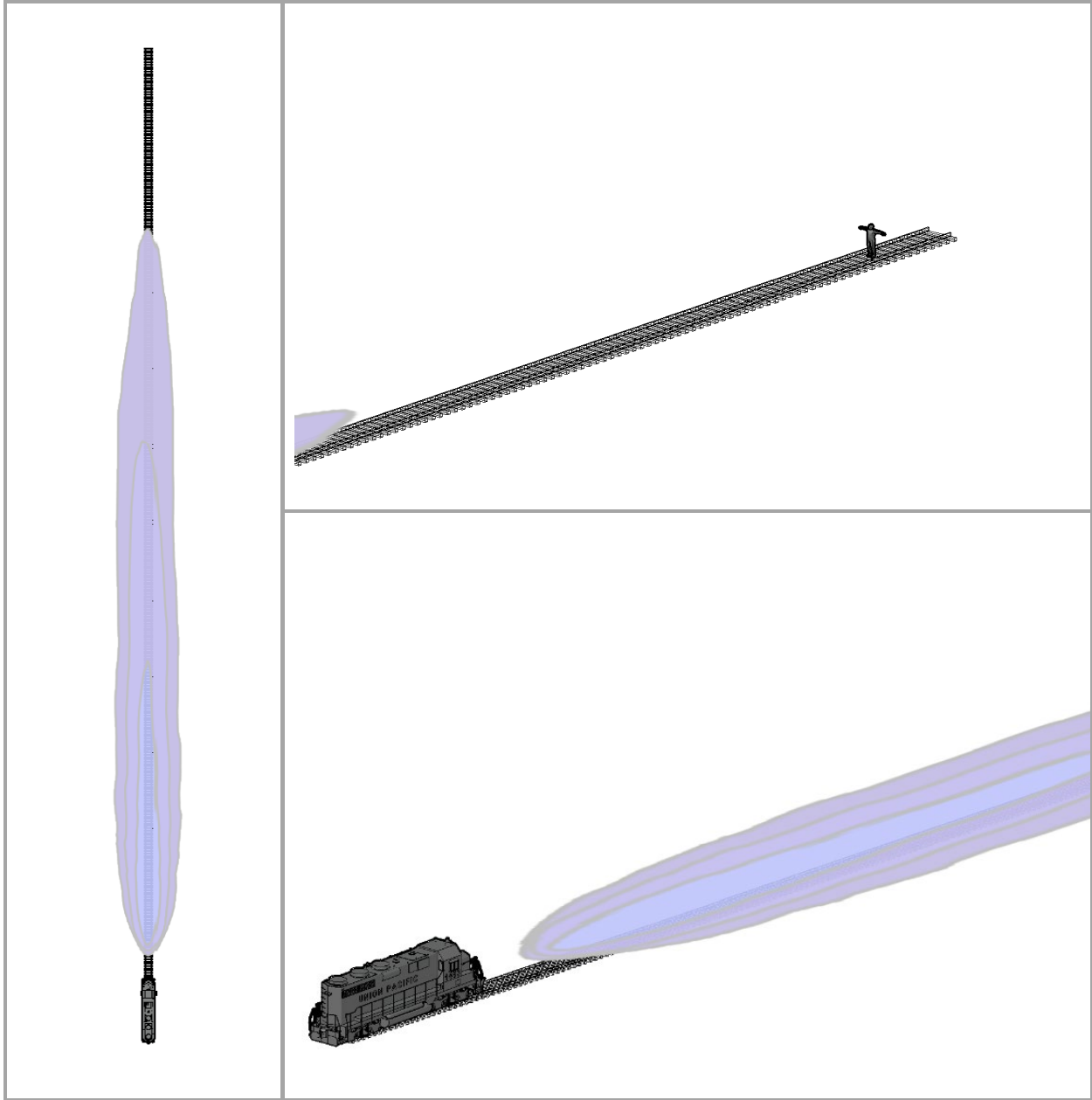
Figure 5. 3-Way View of an Illuminance map for a Smart Light Source dual-lamp headlight (S3 LED). The human figure (upper-right plot) stands 800 ft away from the light source.
