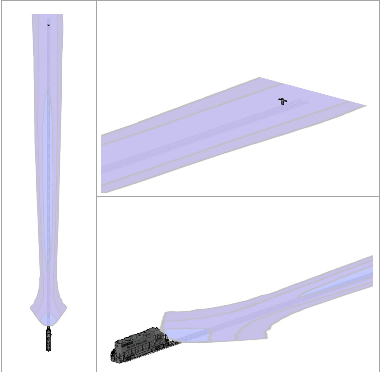
Figure 3. 3-Way View of an Illuminance map for a Hydra-Tech 7000K dual-lamp headlight (S1 LED). The human figure (upper-right plot) stands 800 ft away from the light source.
