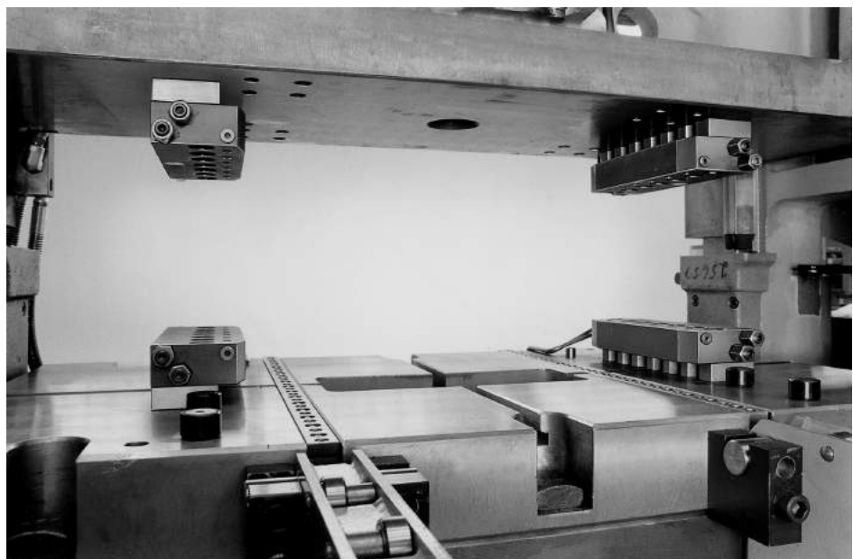
Clamping bars installed in press bed and ram. Easy loading of dies using die change consoles and lateral guide rollers.
