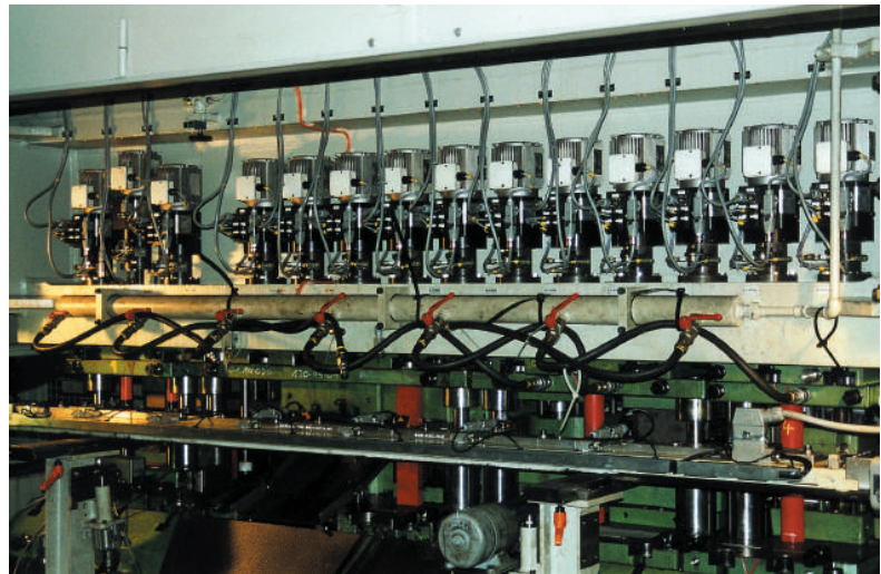
Electromechanical swivel and pull clamping elements mounted on a transfer press.
