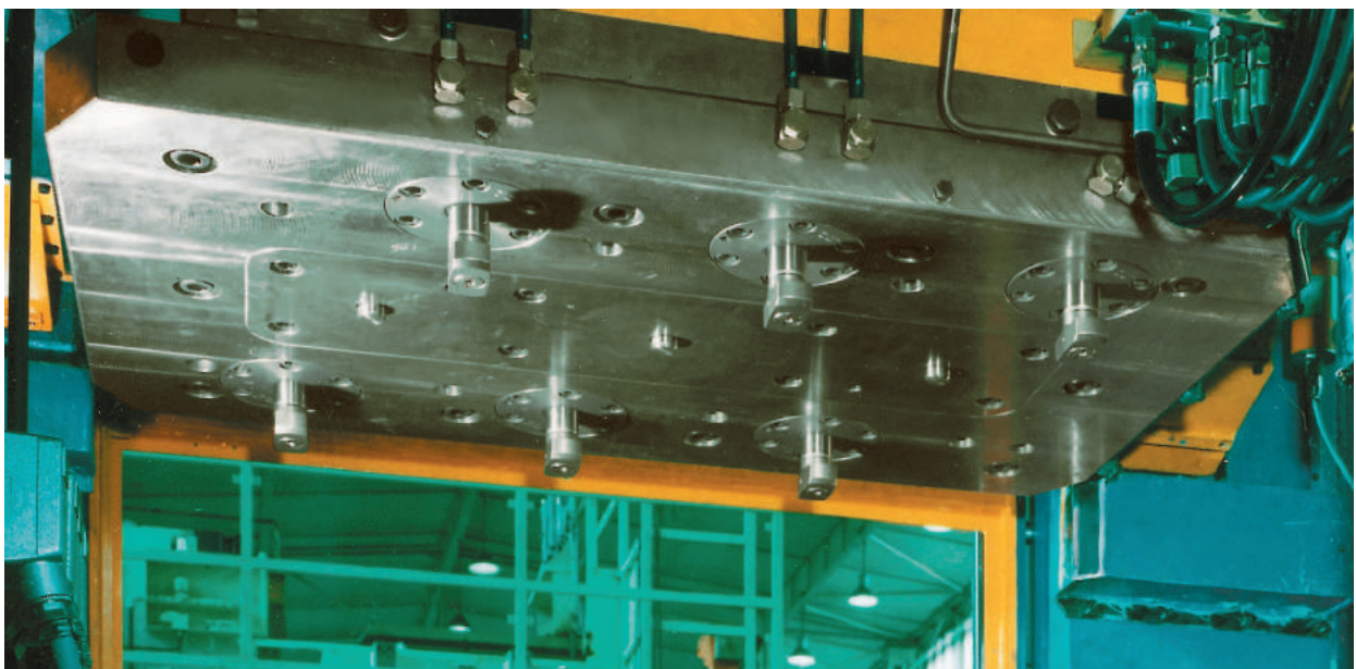
The swing clamps are fastened in the press ram. The ram is in the upper position and the swing clamps are extended (die change position).
