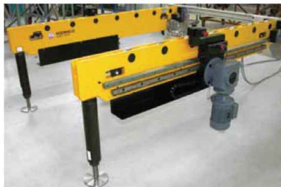
Drive console with motor mounted at the right side Load: 100 kN, length: 2500 mm.
