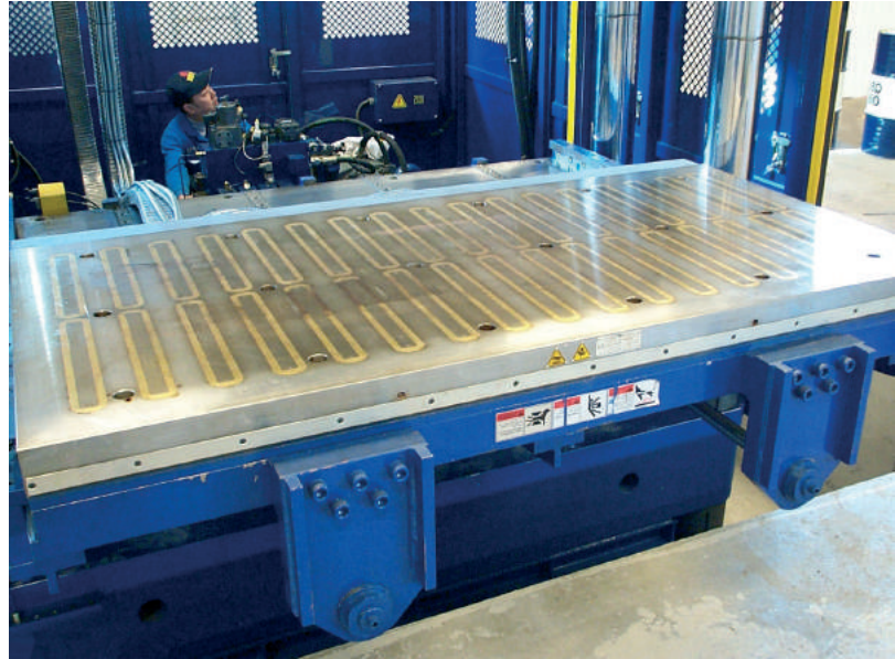
Magnetic clamping system on a vertical press for temperatures up to 240° C
