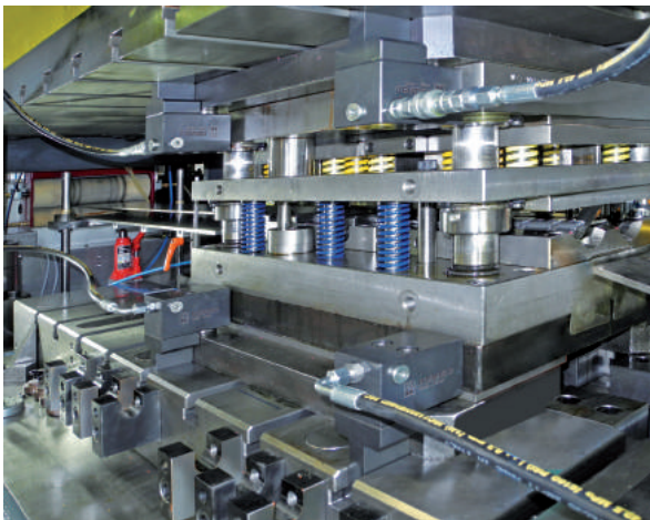
Sliding clamp with T-slot adapter in press bed and ram, roller bars and carrying consoles for tool insertion.
