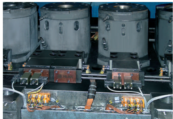
Wedge clamps with flanged directional seat valves. Clamping and unclamping positions are electrically controlled. Little installation work as a result of plug-type connections between the clamps.
