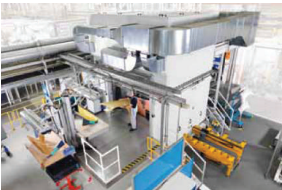
Die changing console with drive and side loading of the press.
