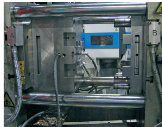
Magnetic clamping system on URPE die casting machine CC 125, closing force 1500 kN, magnetic force 110 kN, temperature range up to 240° C.
