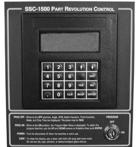
Photo 4.1 Keypad/Display With Program Off/ On Selector Switch
