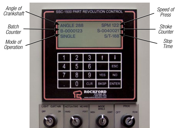
Example of the Main Run Screen on the Keypad/Display With Selector Switches
