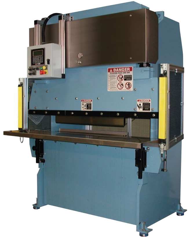
Hydraulic Press Brake With Remote Operator Station
