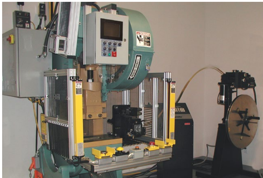
OBI With Press Automation System and Servo Feed Interface
