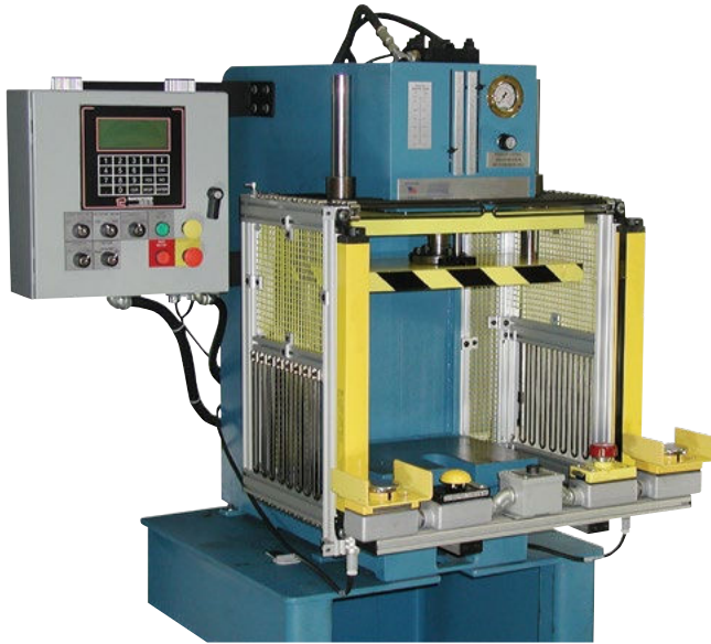
Hydraulic Press With a Light Curtain and Two-Hand Control Device as the Point-of-Operation Safeguard— Also Has a Hydraulic Control With Control Reliability
