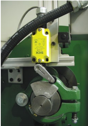
Top-of-Stroke Limit Switch Mounted Above Cam and Strap Assembly on the Crankshaft
