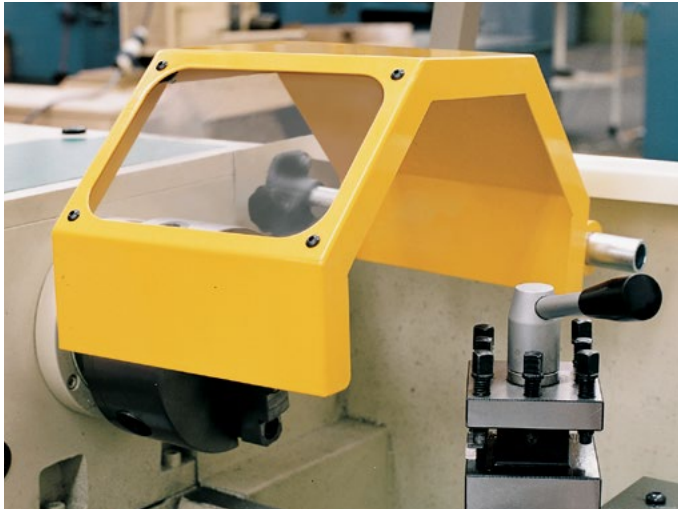
Shield in position. Machine is ready for machining workpiece.
