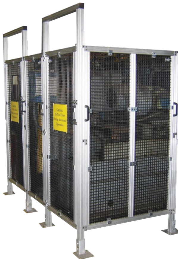
Perimeter Guard Around a Transfer Line
