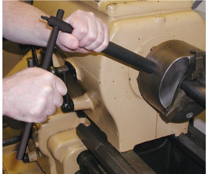
Adjusting the chuck using a long-handled spring-loaded chuck wrench.
