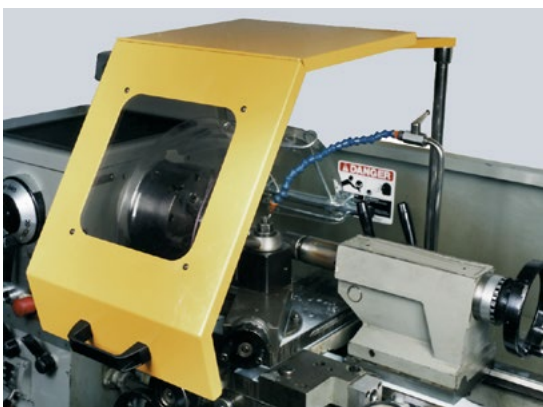
Shield travels with the crossslide for operator protection.
