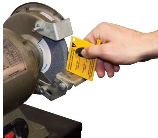
Checking work rest opening.
