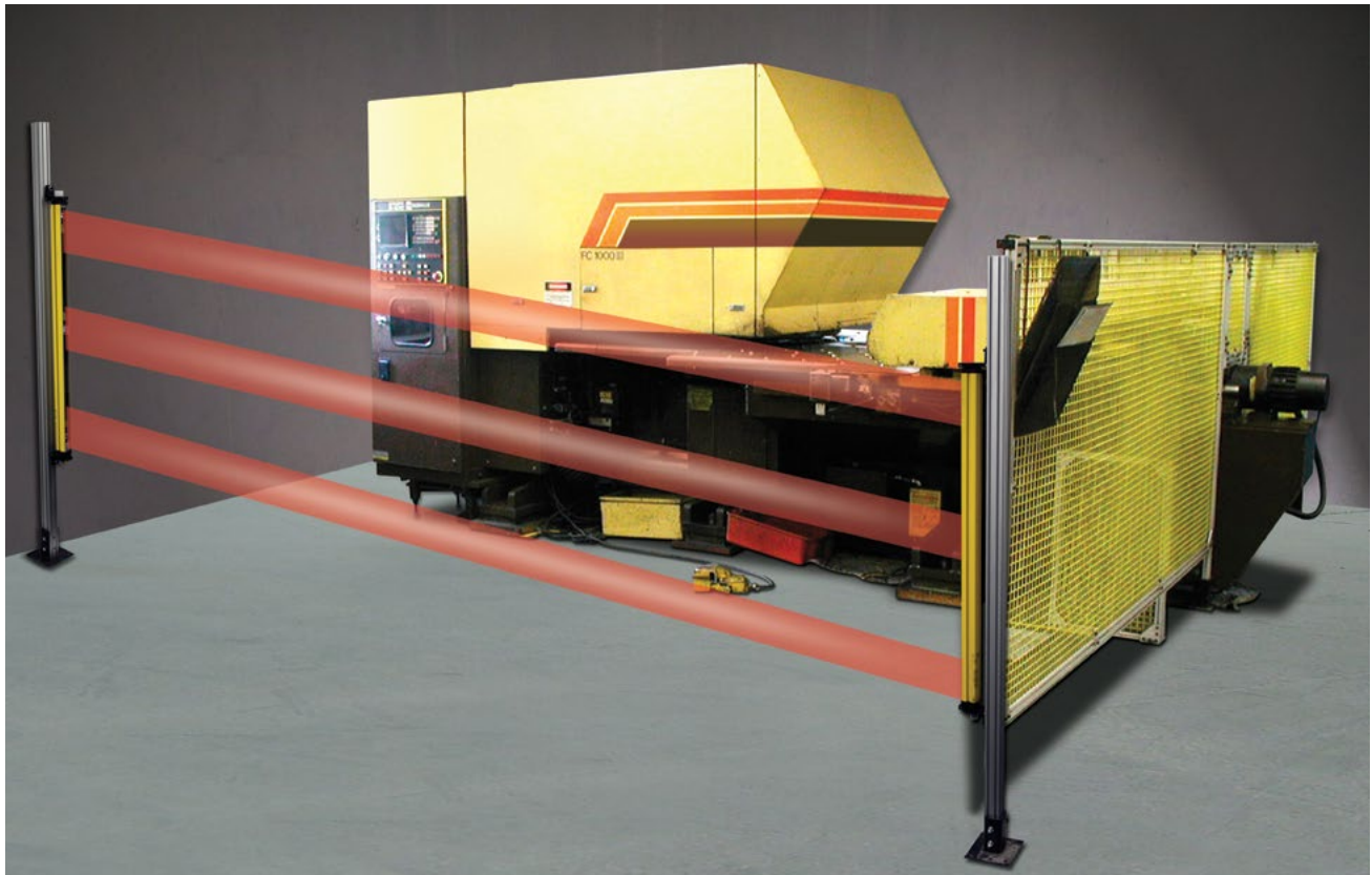
Perimeter Light Curtain System Used as Access Protection for an Automatic Machine Work Envelope
