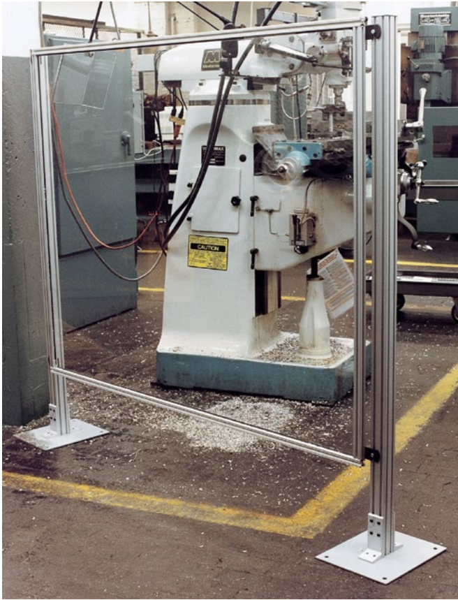
Free-standing shield used to protect the area around a milling machine from flying chips.
