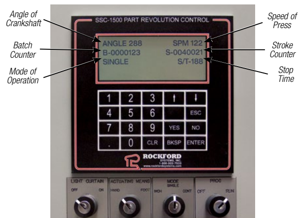
Example of the Main Run Screen on the Keypad/Display With Selector Switches
