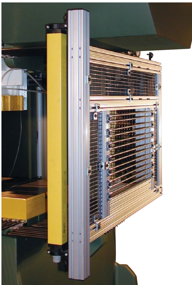
Swing-Away Light Curtain Mounting Bracket with Material Feeding Segment Built Into the Guards
