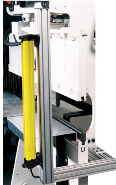
3-Section (OBI) Stationary Light Curtain Mounting Bracket (barrier guard has been removed from machine for photo)
