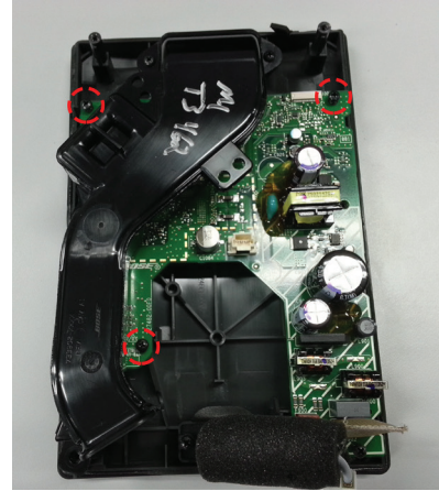
Figure 27. Main PCB, Screws
