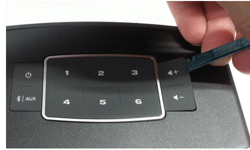
Figure 12. Keypad, Button Pad
