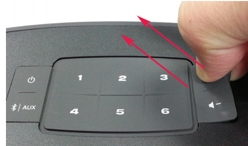
Figure 13. Button Pad, Removal
